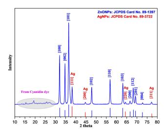
Fig. 5 XRD spectra of Ag-ZnONPs@Cy shows the peaks of each ZnONPs, AgNPs and cyanidin dye.
