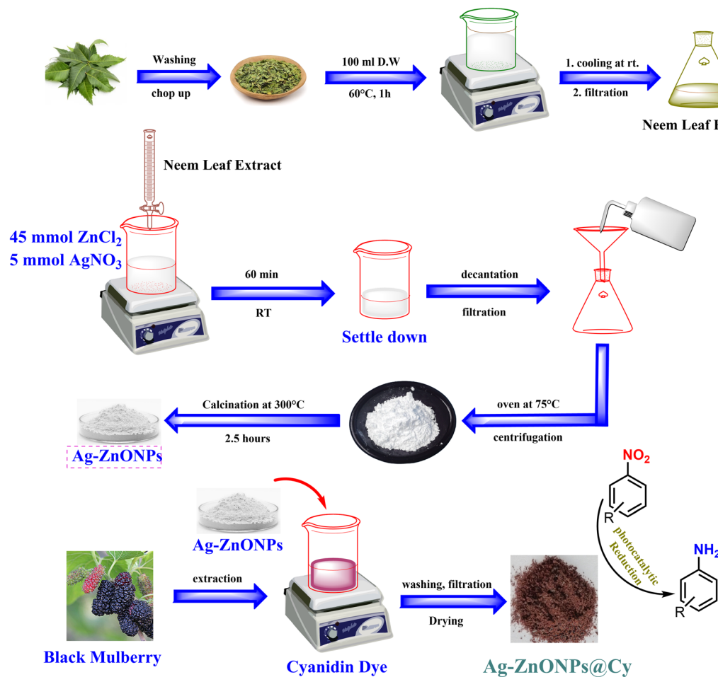
Scheme 1 Illustrative process for producing and utilizing Ag-ZnONPs@Cy, depicted step-by-step.
