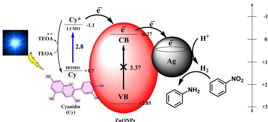
Fig. 9 A proposed mechanism for the reduction of nitroarenes to aminoarenes by Ag-ZnONPs@Cy.
