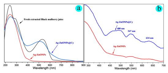
Fig. 6 (a) UV-Vis spectra of fresh extracted black mulberry juice, Ag-ZnONPs and Ag-ZnONPs@Cy, and (b) DRS spectra of Ag-ZnONPs and Ag-ZnONPs@Cy.
