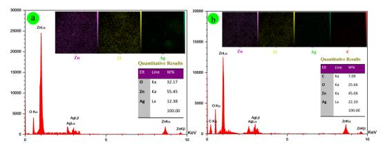
Fig. 3 EDX spectrum and elemental mapping of (a) Ag-ZnONPs, and (b) Ag-ZnONPs@Cy.
