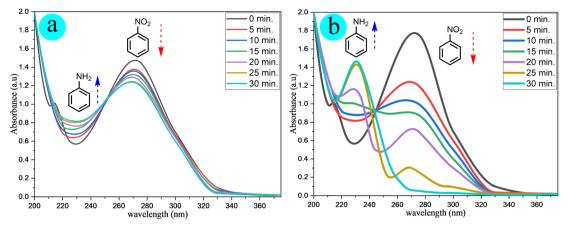
Fig. 7 UV-visible spectra obtained after 30 minutes for the transformation of NB to AN using (a) Ag-ZnONPs and (b) Ag-ZnONPs aCV.
