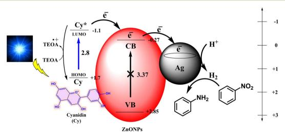
Fig. 9 A proposed mechanism for the reduction of nitroarenes to aminoarenes by Aq-ZnONPs@Cy.
