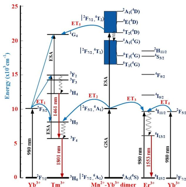
Fig. 6 Energy levels of  $\text{Er}^{3+}$ ,  $\text{Tm}^{3+}$ ,  $\text{Yb}^{3+}$ ,  $\text{Mn}^{2+}$ - $\text{Yb}^{3+}$  dimer and mechanisms of  $\text{ET}_l$  ( $l = 1, 2, 3, 4,$  and  $5$ ) processes in the SZB glass system.
