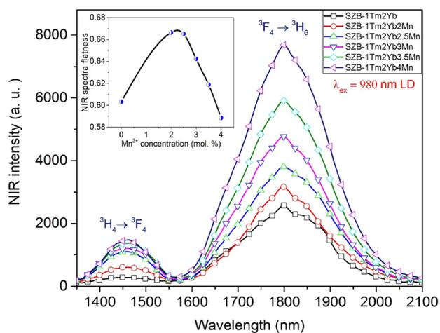
Fig. 5 NIR emission spectra of the SZB-1Tm2YbxMn ( $x = 0, 2, 2.5, 3, 3.5,$  and  $4$  mol%) glass samples.
