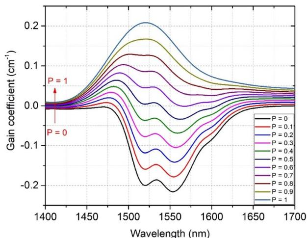
Fig. 12 Gain coefficient for the  ${}^4I_{13/2} \rightarrow {}^4I_{15/2}$  transition of  $\text{Er}^{3+}$  ions in the SZB-0.5Er<sub>2</sub>Yb<sub>2</sub>Mn glass sample.
