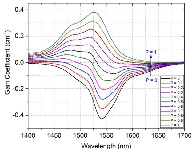
Fig. 10 Gain coefficient for the  ${}^4I_{13/2} \rightarrow {}^4I_{15/2}$  transition of  $\text{Er}^{3+}$  ions in the SZB-0.5Er glass sample.
