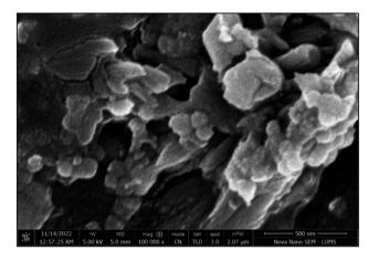
Fig. 11 SEM image of the IA nanoemulsion.
