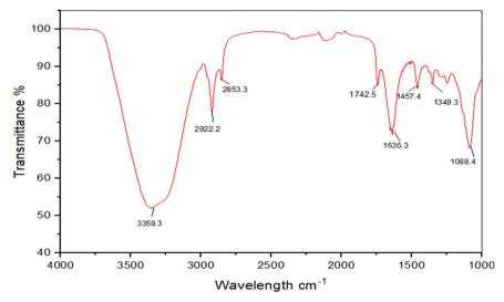
Fig. 10 FT-IR spectrum of the IA-mediated nanoemulsion.
