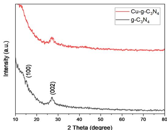
Fig. 2 XRD patterns of g-C<sub>3</sub>N<sub>4</sub> and Cu-g-C<sub>3</sub>N<sub>4</sub>.
