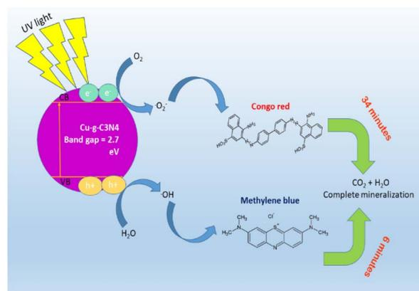
Fig. 24 Schematic diagram for photocatalytic degradation of dyes using Cu-g-C<sub>3</sub>N<sub>4</sub> catalyst.
