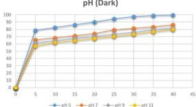
Fig. 19 Effect of pH on degradation of Congo red.
