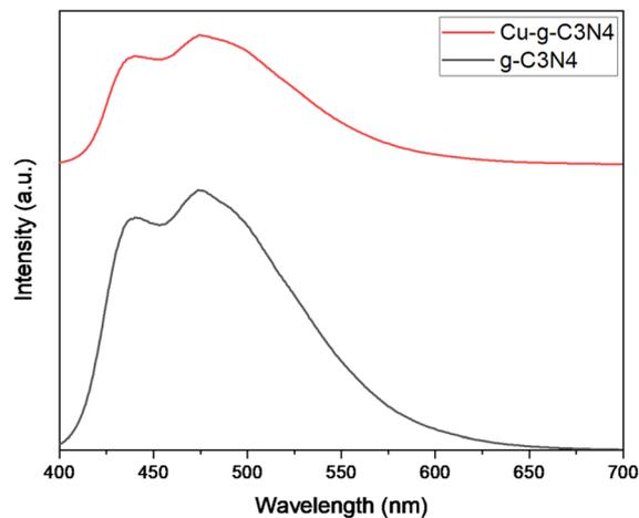
Fig. 8 Photo luminescence spectra of g-C<sub>3</sub>N<sub>4</sub> and Cu-g-C<sub>3</sub>N<sub>4</sub>.
