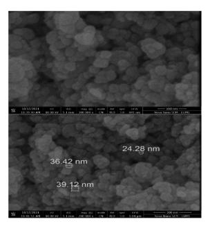
Fig. 3 SEM images of Cu-g-C<sub>3</sub>N<sub>4</sub>.
