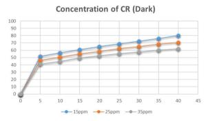
Fig. 17 Effect of concentration of Congo red on its degradation.
