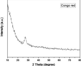
Fig. 22 XRD pattern of Cu-g-C<sub>3</sub>N<sub>4</sub> catalyst after five reaction cycles.
