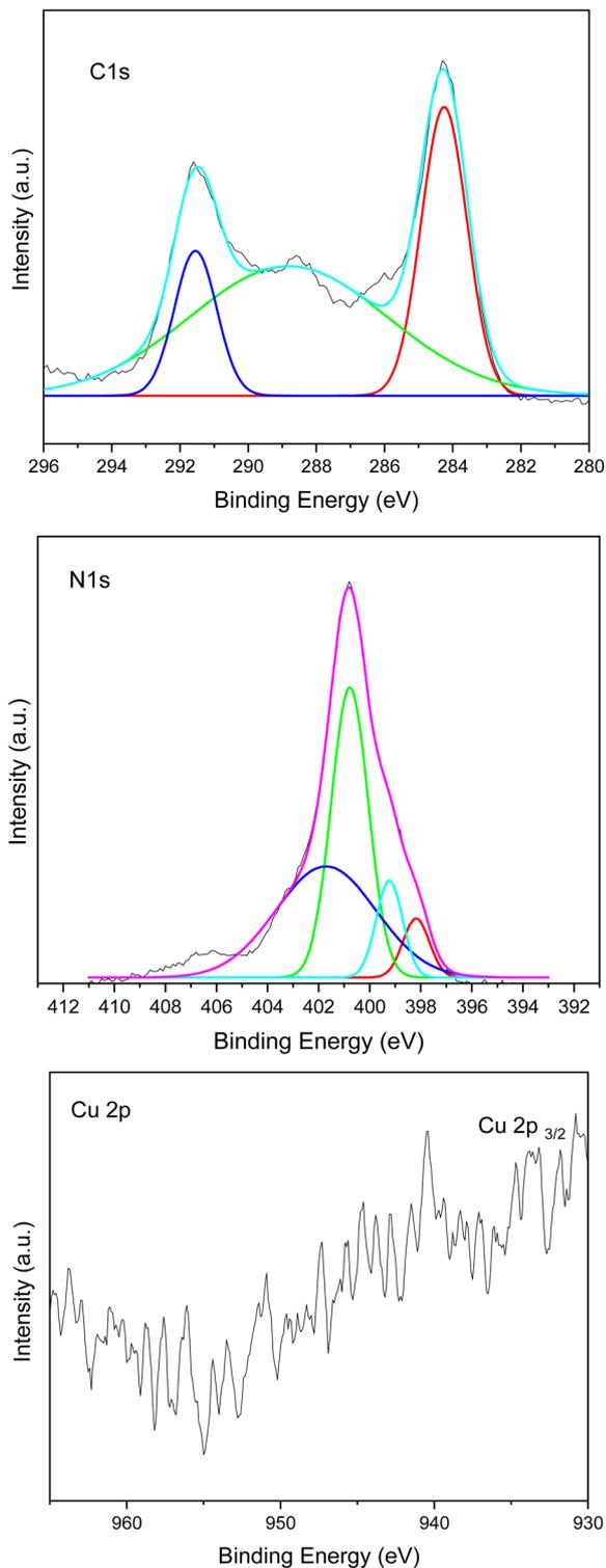
Fig. 7 XPS spectra of Cu-g-C<sub>3</sub>N<sub>4</sub>.
