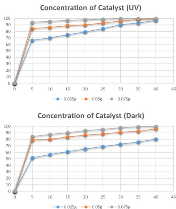
Fig. 18 Effect of dose catalyst on degradation of Congo red.
