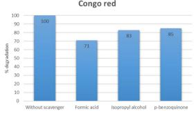
**Fig. 23** Effect of different scavenger on the degradation of methylene blue and Congo red.
