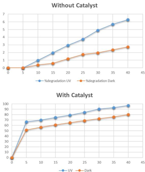
Fig. 16 Effect of time on degradation of Congo red.
