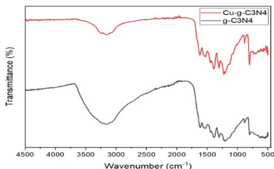
Fig. 5 FTIR spectra of  $g\text{-C}_3\text{N}_4$  and  $\text{Cu-g-C}_3\text{N}_4$ .
