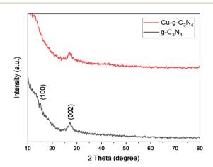
Fig. 2 XRD patterns of  $q-C_3N_4$  and  $Cu-q-C_3N_4$ .
