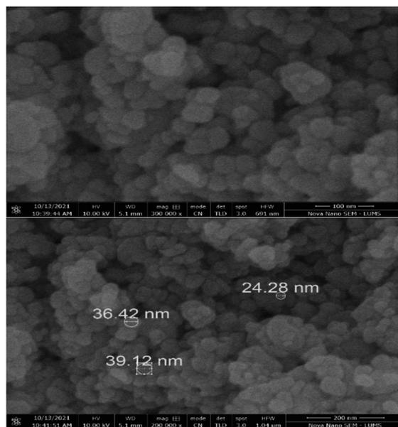
Fig. 3 SEM images of Cu-g-C<sub>3</sub>N<sub>4</sub>.
