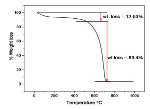
Fig. 6 TGA curve of Cu-g-C<sub>3</sub>N<sub>4</sub>.
