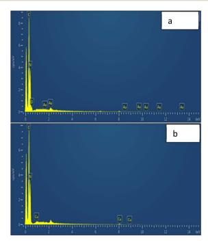
Fig. 4 EDX spectra of (a) g-C<sub>3</sub>N<sub>4</sub> and (b) Cu-g-C<sub>3</sub>N<sub>4</sub>.
