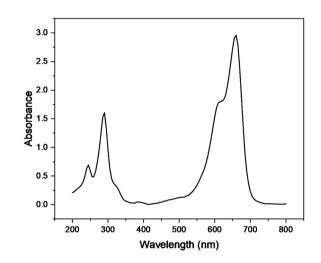
Fig. 9 UV-vis absorption spectra of methylene blue.
