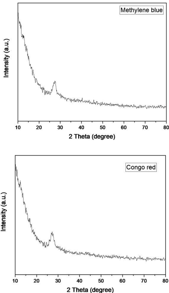
Fig. 22 XRD pattern of Cu-g-C<sub>3</sub>N<sub>4</sub> catalyst after five reaction cycles.
