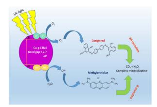
Fig. 24 Schematic diagram for photocatalytic degradation of dyes using  $\text{Cu-g-C}_3\text{N}_4$  catalyst.
