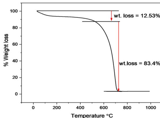
Fig. 6 TGA curve of  $\text{Cu-g-C}_3\text{N}_4$ .
