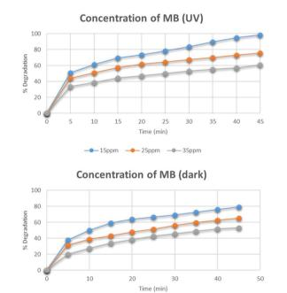
Fig. 11 Effect of concentration of methylene blue on its degradation.
