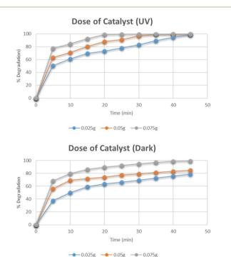
Fig. 12 Effect of dose of catalyst on degradation of methylene blue.
