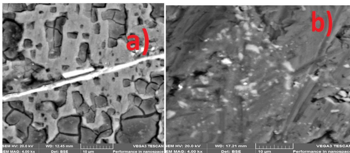
Fig. 9 SEM image of corroded surface (a) mild steel (b) 15 wt% MCAP coated sample.
