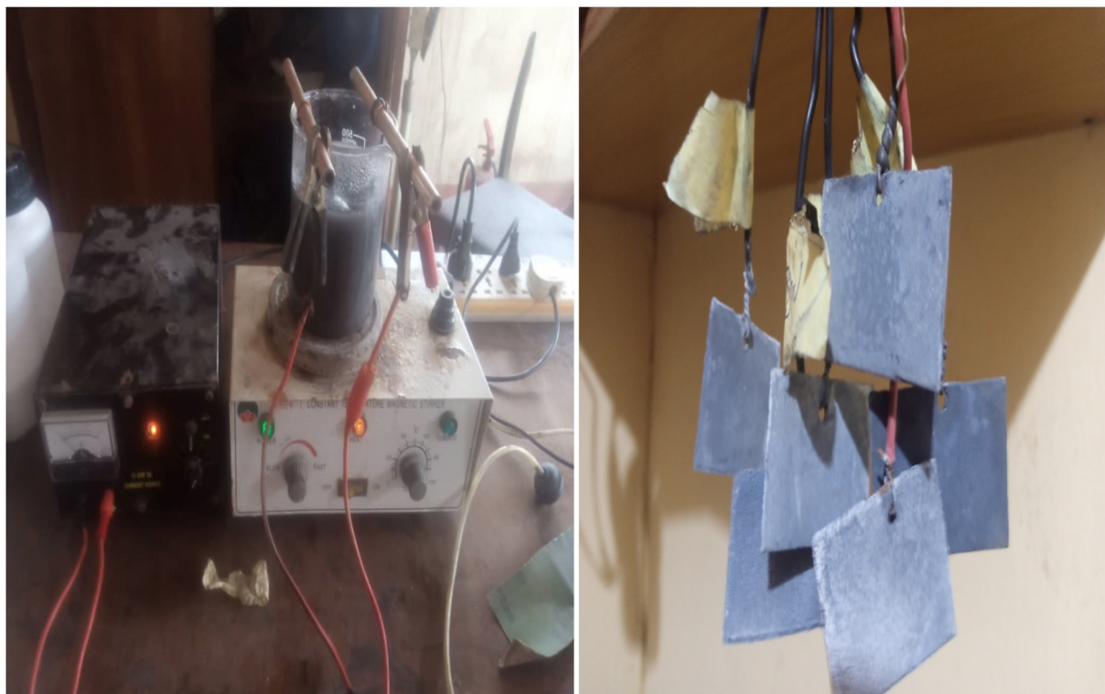
Fig. 1 Photograph of the electrodeposition and produced sample.
