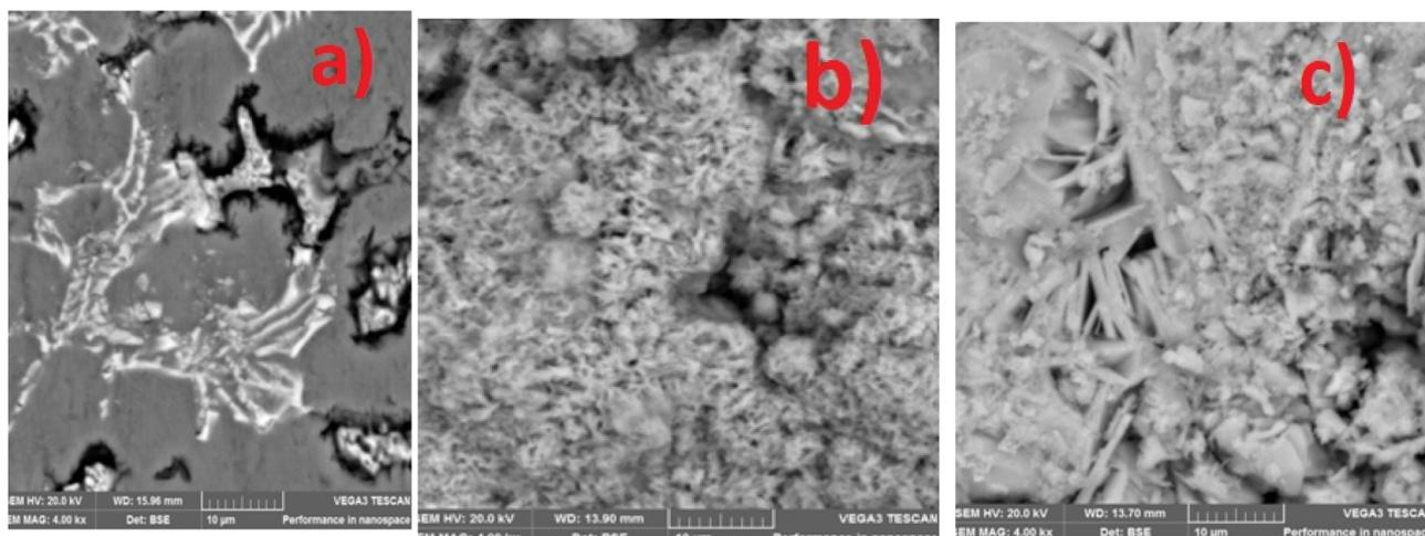
Fig. 3 SEM of the (a) substrate (b) 5 wt% MCAP coated sample (c) 15 wt% MCAP coated sample.
