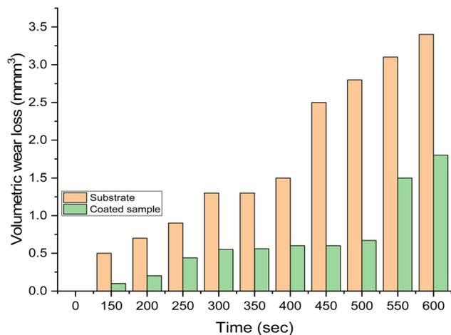
Fig. 10 The volumetric wear rate with time.
