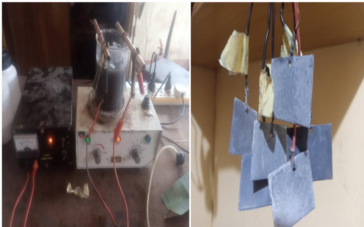
Fig. 1 Photograph of the electrodeposition and produced sample.
