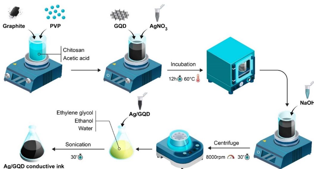
Scheme 1 Synthesis process of conductive AgNPrs-GQDs nano-ink.
