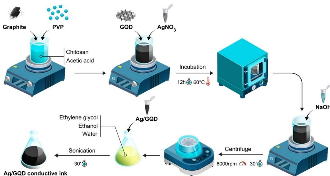
Scheme 1 Synthesis process of conductive AgNPrs-GQDs nano-ink.
