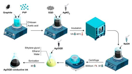
Scheme 1 Synthesis process of conductive AgNPrs-GQDs nano-ink.
