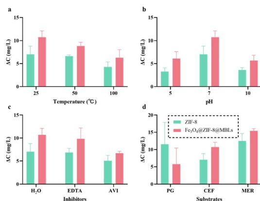
Fig. 4 Change in concentration of CEF (2 mL) degraded by ZIF-8 and  $\text{Fe}_3\text{O}_4@ZIF-8@MBLs$  within 1 h after treatment with different temperatures (a), pH (b), and enzyme inhibitors (c); change in concentration of PG, CEF, and MER (2 mL) degraded by ZIF-8 and  $\text{Fe}_3\text{O}_4@ZIF-8@MBLs$  within 1 h (d).
