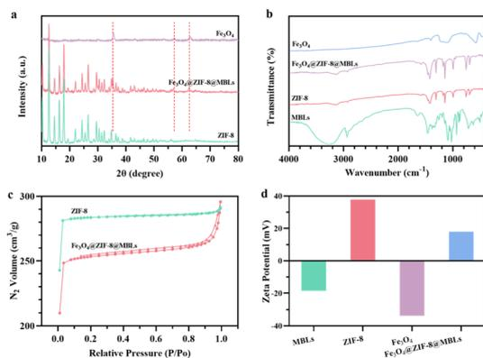
Fig. 2 The XRD patterns (a), FTIR spectra (b),  $\text{N}_2$  adsorption (circles) – desorption (triangles) isotherms (c), and zeta potential (d) of ZIF,  $\text{Fe}_3\text{O}_4@ZIF-8@MBLs$ , and their raw materials.  $P$ , partial pressure of nitrogen.  $P_0$ , saturated vapor pressure of nitrogen.
