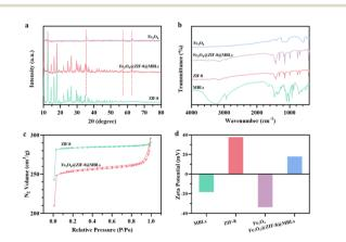
Fig. 2 The XRD patterns (a), FTIR spectra (b), N<sub>2</sub> adsorption (circles) desorption (triangles) isotherms (c), and zeta potential (d) of ZIF, Fe<sub>3</sub>-O4@ZIF-8@MBLs, and their raw materials. P, partial pressure of nitrogen.  $P_0$ , saturated vapor pressure of nitrogen.
