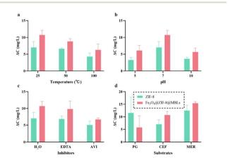
Fig. 4 Change in concentration of CEF (2 mL) degraded by ZIF-8 and  $Fe_3O_4$ @ZIF-8@MBLs within 1 h after treatment with different temperatures (a), pH (b), and enzyme inhibitors (c); change in concentration of PG, CEF, and MER (2 mL) degraded by ZIF-8 and  $Fe_3O_4$ @ZIF-8@MBLs within 1 h (d).
