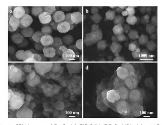
Fig. 1 SEM images of Fe $_3$ O $_4$  (a), ZIF-8 (b), ZIF-8@MBLs (c), and Fe $_3$ -O $_4$ @ZIF-8@MBLs (d).
