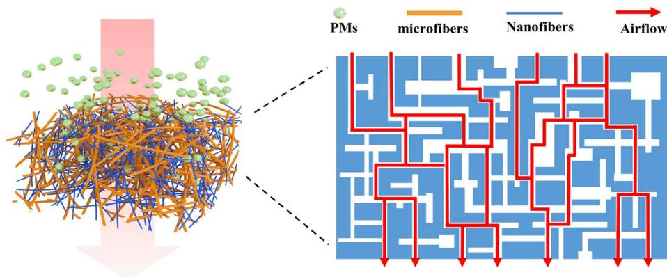
Fig. 7 A schematic explaining the filtration process of CBM for PMs.
