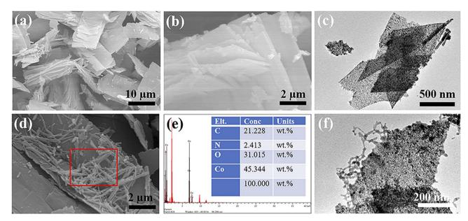
Fig. 6 SEM images of  $Co_3O_4$  at different magnifications: (a) low magnification and (b) high magnification. (c) TEM image of  $Co_3O_4$ . Characterization of PPy@ $Co_3O_4$  catalyst: (d) SEM image, (e) EDS analysis, and (f) TEM image.
