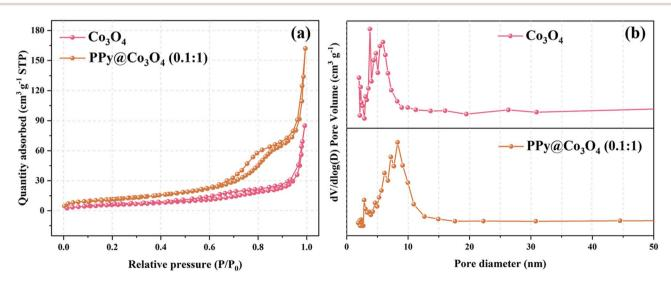
Fig. 4 (a) N<sub>2</sub> adsorption-desorption isotherms and (b) corresponding BJH pore size distribution curves for Co<sub>3</sub>O<sub>4</sub> and PPy@Co<sub>3</sub>O<sub>4</sub>.
