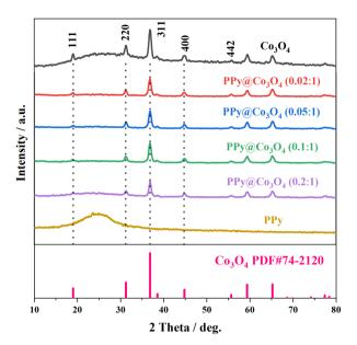
Fig. 2 XRD patterns of the prepared Co<sub>3</sub>O<sub>4</sub>, PPy, and PPy@Co<sub>3</sub>O<sub>4</sub> catalyst samples with different mass ratios.
