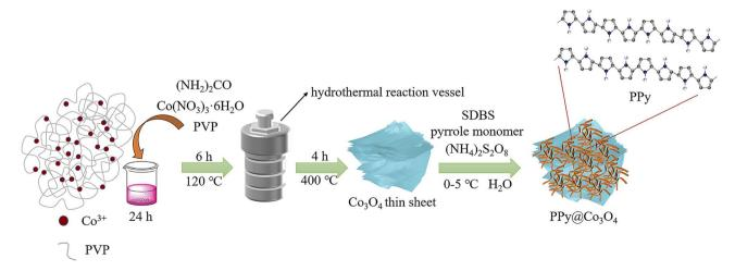
Fig. 1 The preparation process of the PPy@Co<sub>3</sub>O<sub>4</sub> electrocatalyst material.
