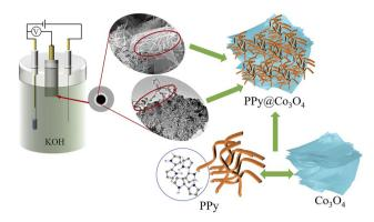
Fig. 10 Mechanism diagram of the PPy@Co<sub>3</sub>O<sub>4</sub> (0.1:1) catalyst.
