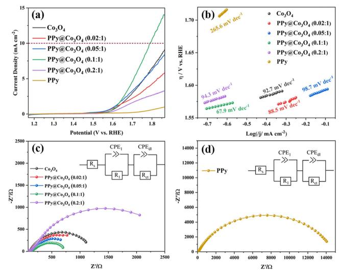
Fig. 7 (a) OER polarization curves of catalysts obtained in 0.1 M KOH solution with a scan rate of 5 mV s $^{-1}$ . (b) Tafel plots. Electrochemical impedance spectra (EIS) for (c) Co<sub>3</sub>O<sub>4</sub> and PPy@Co<sub>3</sub>O<sub>4</sub> and (d) PPy.
