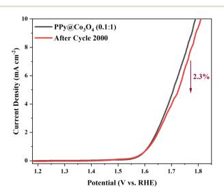
Fig. 9 OER stability test of PPy@Co<sub>3</sub>O<sub>4</sub> (0.1:1).
