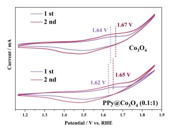
Fig. 8 Pseudocapacitive behavior at first and second cycles during CV test for  $PPy@Co_{\pi}O_4$  (0.1:1).
