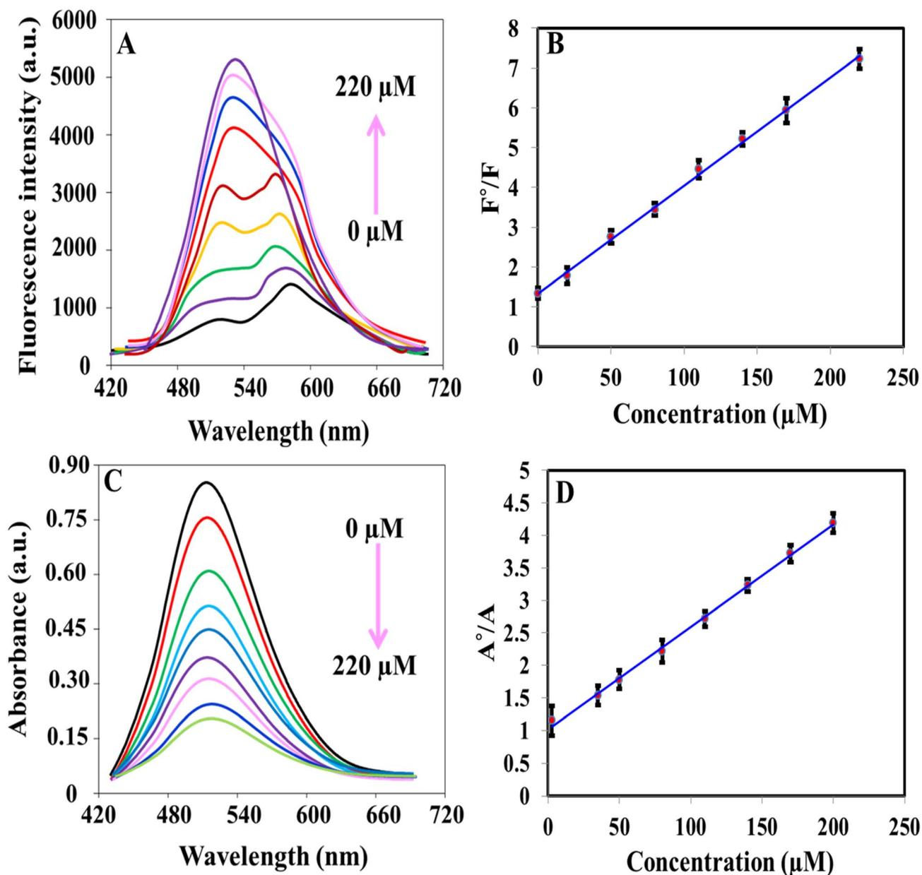
Fig. 4 (A) Fluorescence spectra of iron(II)-ortho-phenanthroline/N, S@g-CDs system in the presence of different concentrations of  $\text{ClO}^-$  (0–220  $\mu\text{M}$ ); (B) calibration plot of  $F^\circ/F$  versus concentration of  $\text{ClO}^-$ ; (C) absorbance spectra of iron(II)-ortho-phenanthroline/N, S@g-CDs system in the presence of different concentrations of  $\text{ClO}^-$  (0–200  $\mu\text{M}$ ); (D) calibration plot of  $A^\circ/A$  versus concentration of  $\text{ClO}^-$ .
