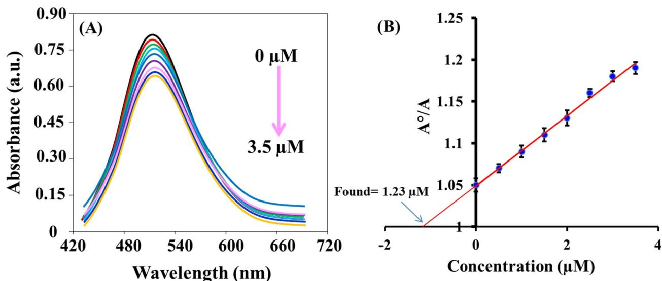
Fig. 6 (A) Absorption spectra of iron(II)-ortho-phenanthroline/N, S@g-CDs system in water sample and in the presence of different concentrations of  $\text{ClO}^-$  (0–3.5  $\mu\text{M}$ ); (B) the standard addition plot for the determination between  $A^\circ/A$  versus the concentration of  $\text{ClO}^-$ .
