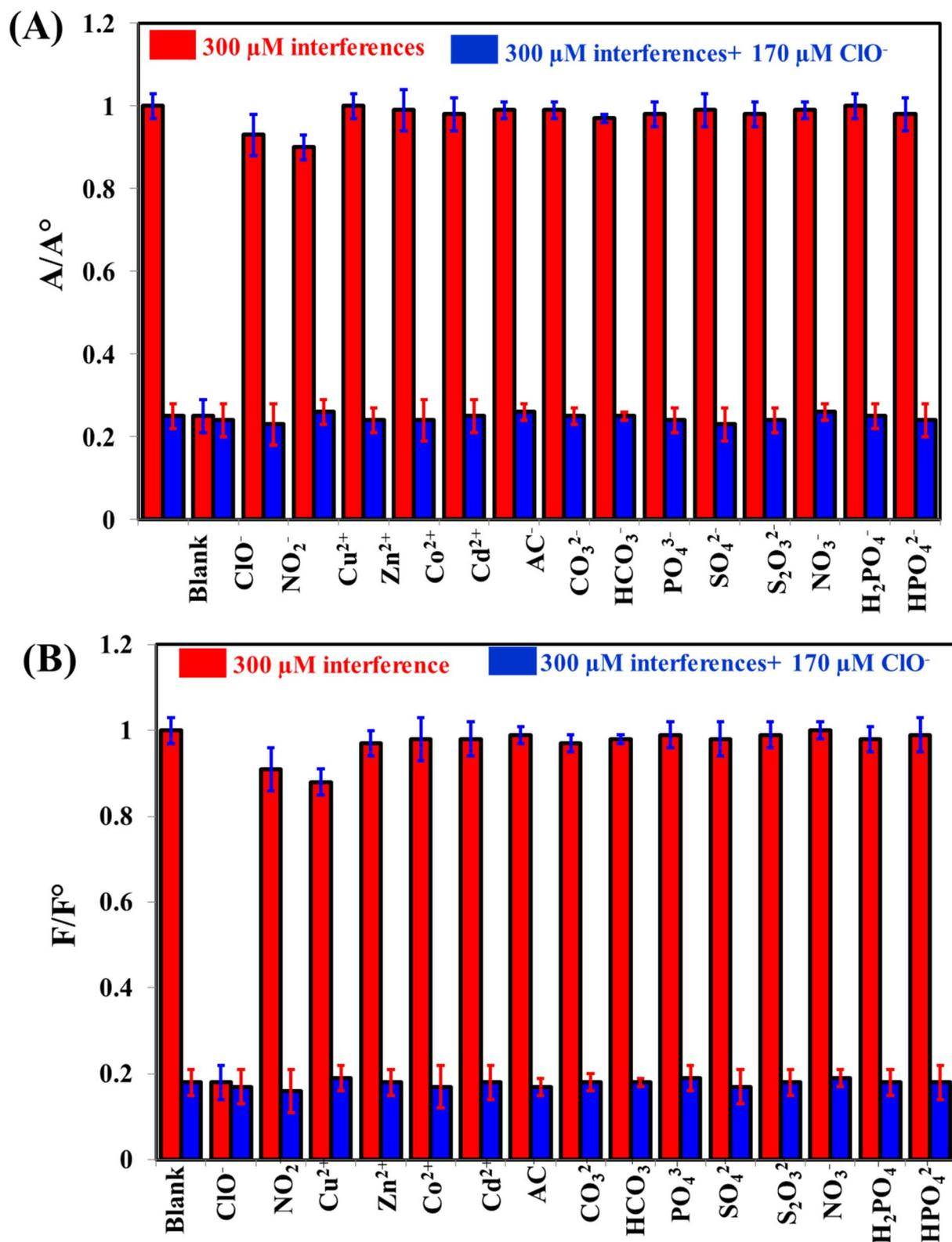
Fig. 5 The selectivity of iron(II)-ortho-phenanthroline/N, S@ $\gamma$ -CDs for the detection of  $170 \mu\text{M ClO}^-$  in the presence of  $300 \mu\text{M}$  interfering species either colorimetrically (A) or fluorometrically (B).
