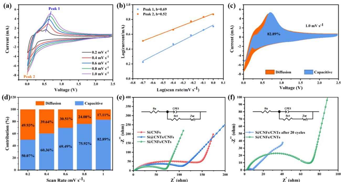
Fig. 8 (a) CV curves of the Si/CNFs/CNTs electrode at various scan rates from 0.2–1.0  $\text{mV s}^{-1}$ ; (b)  $\log(i)/\log(v)$  plots of Si/CNFs/CNTs the electrode at various scan rates from 0.2 to 1.0  $\text{mV s}^{-1}$ ; (c) capacitive contribution at 1.0  $\text{mV s}^{-1}$ ; (d) the percentages of capacitive contributions at various scan rate; (e) Nyquist plots of Si/CNFs, Si@CNTs/CNFs and Si/CNFs/CNTs; (f) Nyquist plots of Si/CNFs/CNTs before and after 20 cycles.
