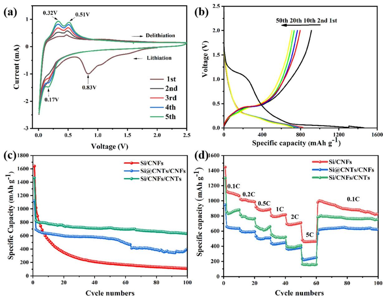
**Fig. 7** (a) CV curves of Si/CNFs/CNTs at first five cycles, (b) charge–discharge curve of Si/CNFs/CNTs at different cycles, (c) cycling performance at 100 mA g<sup>-1</sup> and (d) rate performance of Si/CNFs, Si@CNTs/CNFs and Si/CNFs/CNTs.
