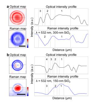
Fig. 2 Relationship between Raman intensity of microlens and optical interference. Top-view false-color optical image of LiCl microlenses (top) and Raman intensity map of Si peak at 520 cm<sup>-1</sup> from the lenses (bottom) on silicon substrates with (a) 300 nm SiO<sub>2</sub> and (b) 150 nm SiO<sub>2</sub>. Shown on the right are intensity profiles along the dotted lines. Scale bars: 3 µm.
