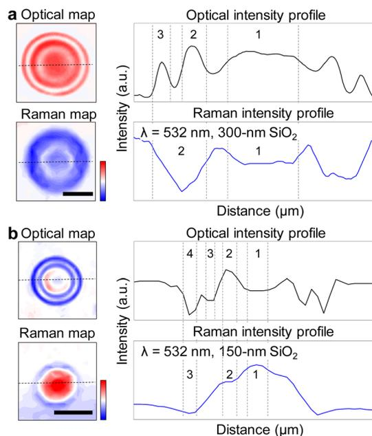
Fig. 2 Relationship between Raman intensity of microlens and optical interference. Top-view false-color optical image of LiCl microlenses (top) and Raman intensity map of Si peak at 520 cm<sup>-1</sup> from the lenses (bottom) on silicon substrates with (a) 300 nm SiO<sub>2</sub> and (b) 150 nm SiO<sub>2</sub>. Shown on the right are intensity profiles along the dotted lines. Scale bars: 3 μm.
