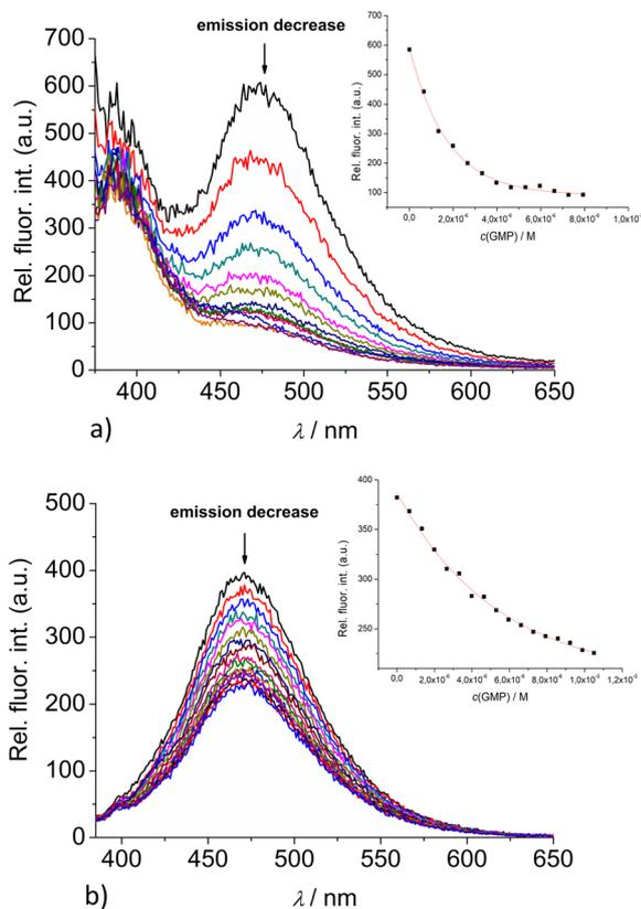
**Fig. 4** Changes in the fluorescence spectra of: (a) **2** ( $c = 5 \times 10^{-7}$  M) and (b) **3** ( $c = 1 \times 10^{-6}$  M), upon titration with GMP ( $c = 1 \times 10^{-3}$  M) at  $\lambda_{\text{exc}} = 350$  nm. (Insets) Dependence of **2** and **3** emission intensity at 475 nm on  $c(\text{GMP})$ . Done at pH 7.0, sodium cacodylate buffer,  $I = 0.05$  M.
