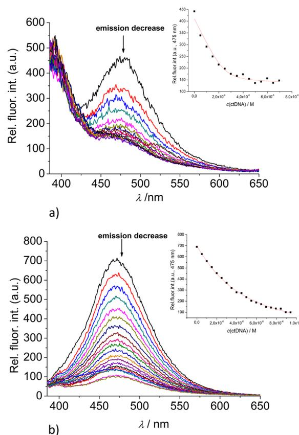
**Fig. 5** Changes in the fluorescence spectra of: (a) **2** ( $c = 5 \times 10^{-7}$  M) and (b) **3** ( $c = 5 \times 10^{-7}$  M) upon titration with ctDNA ( $c = 1 \times 10^{-3}$  M) at  $\lambda_{\text{exc}} = 350$  nm. (Insets) Dependence of **2** and **3** emission intensity at 475 nm on  $c(\text{ctDNA})$ . Done at pH 7.0, sodium cacodylate buffer,  $I = 0.05$  M.
