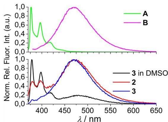
Fig. 2 (Top) 1-pyrenebutyric acid A ( $\lambda_{\text{exc}} = 342$  nm) and peptide B ( $\lambda_{\text{exc}} = 352$  nm) in water (0.01% DMSO). (Bottom) Normalised fluorescence spectra of 2 ( $\lambda_{\text{exc}} = 352$  nm, water), 3 ( $\lambda_{\text{exc}} = 350$  nm, water) and 3 ( $\lambda_{\text{exc}} = 350$  nm, DMSO). Normalisation was performed by dividing a complete spectrum by the maximal intensity of emission.
