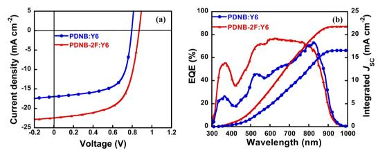
Fig. 5 J-V characteristics (a) and EQE spectra (b) for copolymer: Y6-based NF-PSCs.
