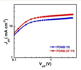
Fig. 6  $J_{\rm ph}$ - $V_{\rm eff}$  curves of PDNB:Y6 and PDNB-2F:Y6-based devices.
