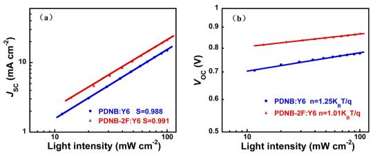
Fig. 7  $P_{\text{light}}$  versus  $J_{\text{SC}}$  (a) and  $V_{\text{OC}}$  (b) of PDNB:Y6 and PDNB-2F:Y6-based devices.
