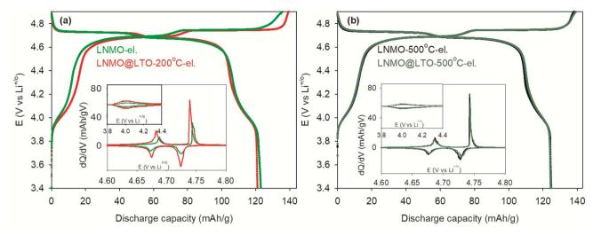
Fig. 8 Initial cycle capacity curves (following cyclic voltammetry) measured at 0.05C, room temperature, in CC-CV (CV at 4.9 V for 30 minutes. CV at  $3.4\,\mathrm{V}$  until the measured current is less than 10% of the initial value) and corresponding  $\mathrm{d}Q/\mathrm{d}V$  plots, for (a) LNMO-el., LNMO@LTO-200 °Cel. and (b) LNMO-500 °C-el., LNMO@LTO-500 °C-el.
