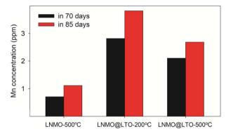
Fig. 11 Mn concentration detected via ICP-AES in 1.0 M LiPF<sub>6</sub> EC/DEC (1:1, v/v) battery electrolyte after dispersion of LNMO-500 °C, LNMO@LTO-200 °C and LNMO@LTO-500 °C powders for 70 or 85 days.
