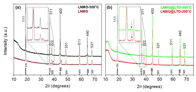
Fig. 2 XRD diffractograms of (a) bare LNMO without (LNMO) and with (LNMO-500 °C) a 500 °C anneal, (b) LTO surface modified LNMO without (LNMO@LTO-200 °C) and with (LNMO@LTO-500 °C) a 500 °C anneal. Reference marks indicate the LiNi<sub>0.5</sub>Mn<sub>1.5</sub>O<sub>4</sub> phase (PDF 80-2162). Peaks from the Al substrate holder are marked with \*. The two vertical arrows in (b) inset point to the impurity phase.
