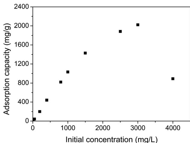
Fig. 9 Adsorption capacity at various initial CV concentrations of a chitosan-based P(AA-co-AMPS) hydrogel with an AA-AMPS ratio of 10 : 1. (Dose = 0.05 g/50 mL, ambient temperature, contact time = 24 h, unadjusted pH).
