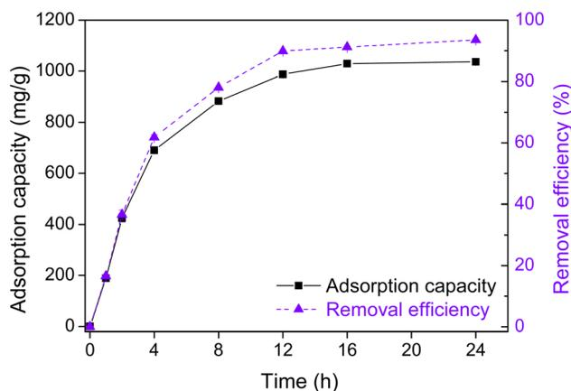
Fig. 6 Adsorption of CV at various contact times of a chitosan-based P(AA-co-AMPS) hydrogel with an AA-AMPS ratio of 10:1. ( $C_o = 1000 \text{ mg L}^{-1}$ , dose = 0.05 g/50 mL, ambient temperature, unadjusted pH).
