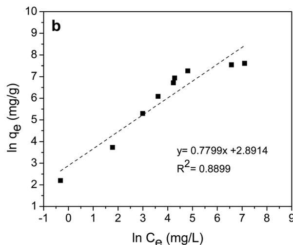
Fig. 10 Linear Langmuir isotherm (a) and linear Freundlich isotherm (b) of CV adsorption of a chitosan-based P(AA-co-AMPS) hydrogel with an AA-AMPS ratio of 10 : 1. (Dose = 0.05 g/50 mL, ambient temperature, contact time = 24 h, unadjusted pH).
