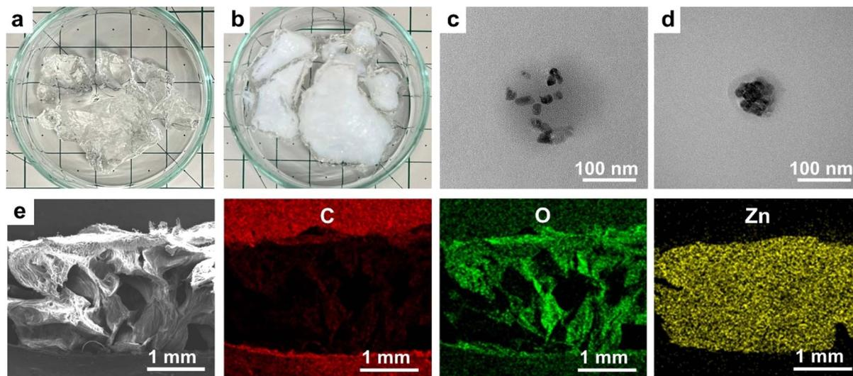
Fig. 11 Photographs of (a) 10 : 1 hydrogel and (b) ZnO/10 : 1 hydrogel composite, (c) and (d) TEM micrographs (magnification 150k $\times$ ) of ZnO particles, and (e) SEM-EDS cross-section micrograph and the corresponding elemental maps of ZnO/10 : 1 hydrogel composite.
