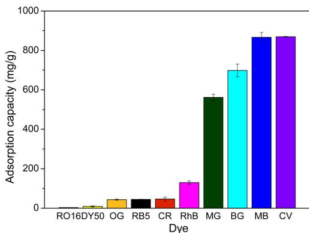
Fig. 4 Adsorption capacity of chitosan-based P(AA-co-AMPS) hydrogel with an AA-AMPS ratio of 5:1 towards various anionic and cationic dyes. ( $C_o = 1000 \text{ mg L}^{-1}$ , dose = 0.05 g/50 mL, ambient temperature, contact time = 24 h, unadjusted pH).
