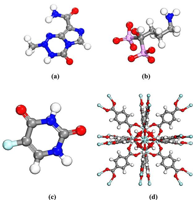
Fig. 7 Equilibrium geometries of (a) TMZ, (b) Ald, (c) 5-FU and (d) UiO-66 by Dmol<sup>3</sup> module in Materials Studio 2017. Colored balls represent O in red, C in gray, N in blue, F of 5-FU in light green and H in white.
