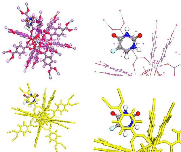
Fig. 10 5-FU adsorption on UiO-66 adsorbent in gas phase.
