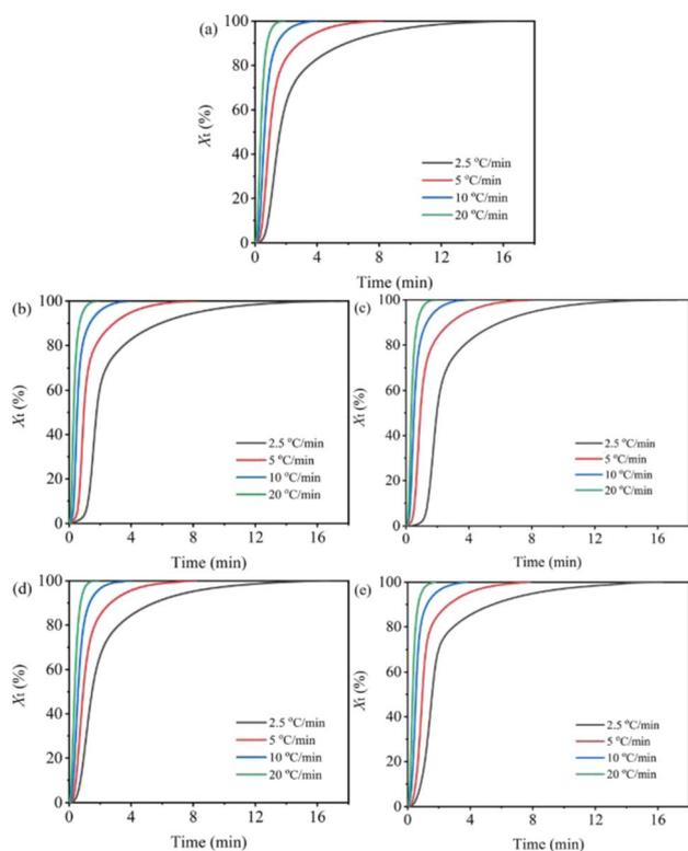
Fig. 3 Relative degree of crystallinity versus time for non-isothermal crystallization of samples at different cooling rates: (a) H/U, (b) H/U<sub>2</sub>, (c) H/U<sub>10</sub>, (d) H/U<sub>2</sub>-S, (e) H/U<sub>10</sub>-S.
