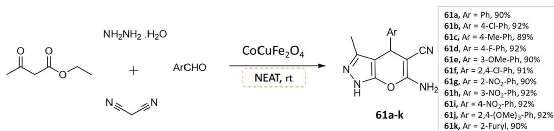
Scheme 61 Synthesis of pyrano[2,3-c]pyrazole derivatives in solvent-free conditions using CoCuFe<sub>2</sub>O<sub>4</sub> nanocrystals.
