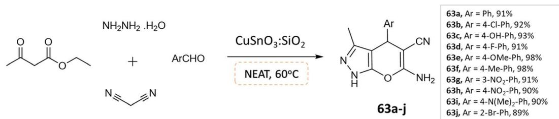
Scheme 63 Synthesis of pyrano[2,3-c]pyrazole derivatives in solvent-free conditions using CuSnO<sub>3</sub>:SiO<sub>2</sub> catalyst.
