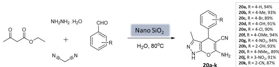
Scheme 20 Nano SiO 2 catalyzed synthesis of pyranopyrazole derivatives in aqueous medium.
