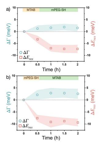
Fig. 5 Localised surface plasmon resonance broadening ( $\Delta \Gamma$ ) and peak shift ( $\Delta E_{res}$ ) of gold nanoprisms obtained applying sequential addition of different thiol types: 10 μM MTAB/100 μM mPEG-SH (a) and 100 μM mPEG-SH/10 μM MTAB (b).
