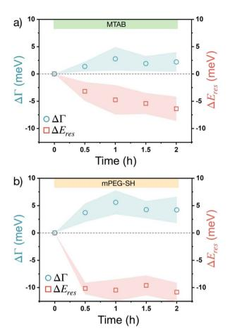
Fig. 4 Localised surface plasmon resonance broadening ( $\Delta \Gamma$ ) and peak shift ( $\Delta E_{res}$ ) of gold nanoprisms obtained by the surface adsorption of different thiol molecules: 10  $\mu$ M MTAB (a) and 100  $\mu$ M mPEG-SH (b).
