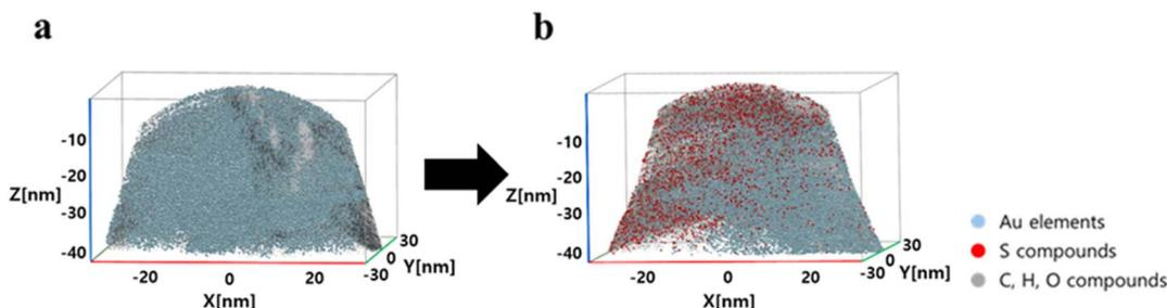
Fig. 6 Associated 3D chemical map of the volume containing a partial section of (a) AuNUs and (b) AuNUs- $\text{H}_2\text{S}$  (pH 4.0,  $25\text{ }^\circ\text{C}$ , and  $20\text{ mM NaCl}$ ) at near-atomic resolution.
