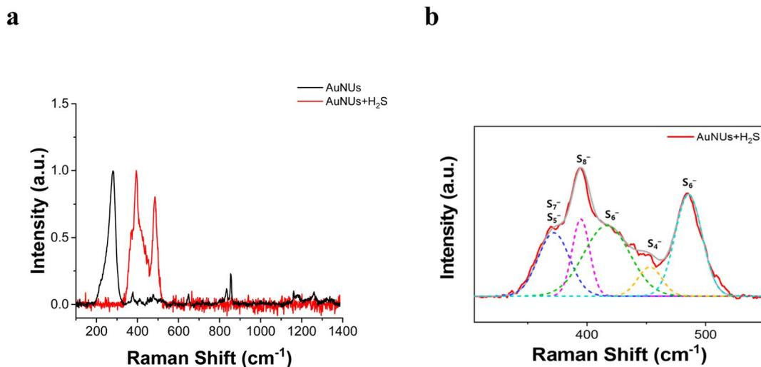
Fig. 3 (a) SERS spectra of AuNUs (black) and AuNUs-H<sub>2</sub>S (red) in the Raman shift range 100–1400 cm<sup>-1</sup> at pH 4.0 and 25 °C in 20 mM NaCl. (b) Deconvoluted Raman peaks with five resolved peaks using the LabSpec 4.16 software. These resolved peaks appear to correspond to oligomeric sulfides S<sub>4</sub><sup>-</sup>, S<sub>5</sub><sup>-</sup>, S<sub>6</sub><sup>-</sup>, S<sub>7</sub><sup>-</sup>, and S<sub>8</sub><sup>-</sup>.
