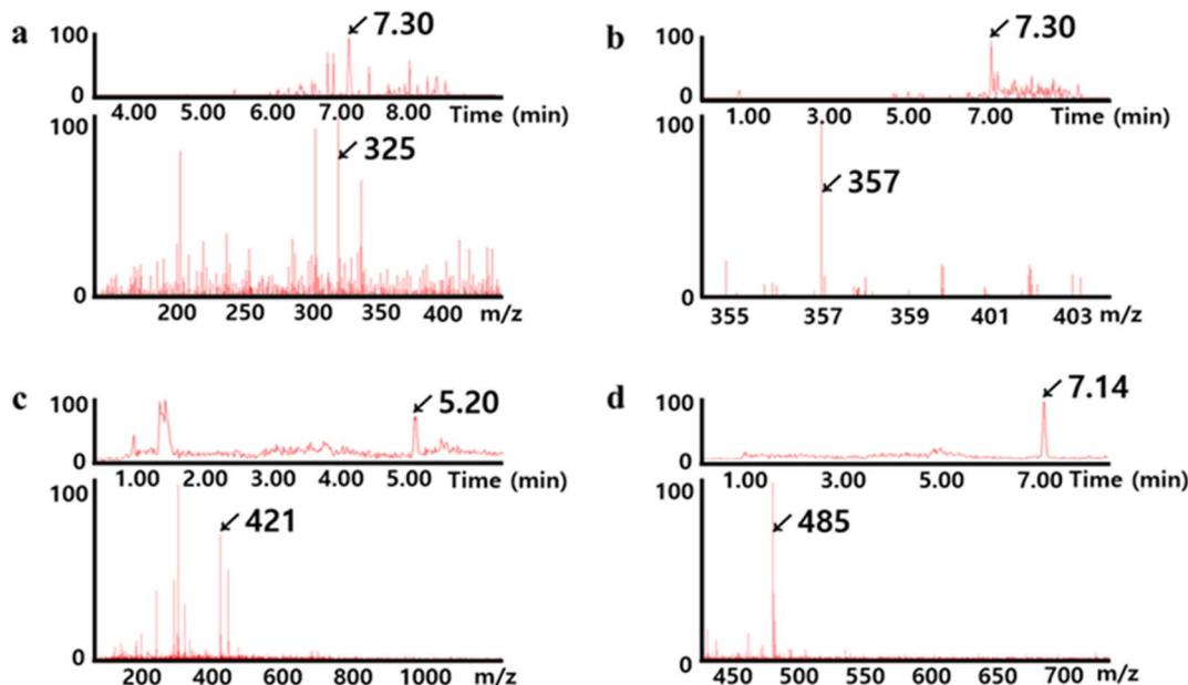
Fig. 5 LC chromatograms (above) and MS spectra (below) for (a)  $\text{AuS}_4^-$ , (b)  $\text{AuS}_5^-$ , (c)  $\text{AuS}_7^-$ , and (d)  $\text{AuS}_9^-$  showing  $\text{Au-S}_n^-$  associated with the oligomeric sulfide coated on the surface of AuNUs.
