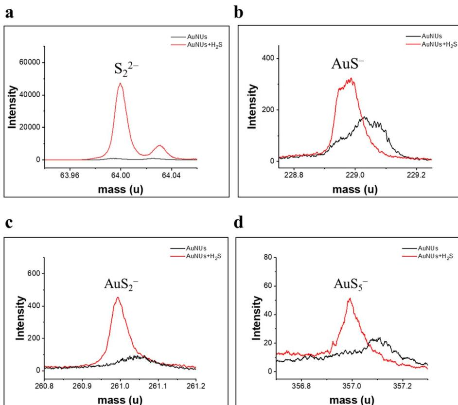
Fig. 4 TOF-SIMS spectra showing characteristic fragments (red) of (a) S<sub>2</sub><sup>2-</sup>, (b) AuS<sup>-</sup>, (c) AuS<sub>2</sub><sup>-</sup>, and (d) AuS<sub>5</sub><sup>-</sup> associated with oligomeric sulfide coated on the surface of AuNUs in the presence of H<sub>2</sub>S and characteristic fragments (black) of AuNUs in the absence of H<sub>2</sub>S.
