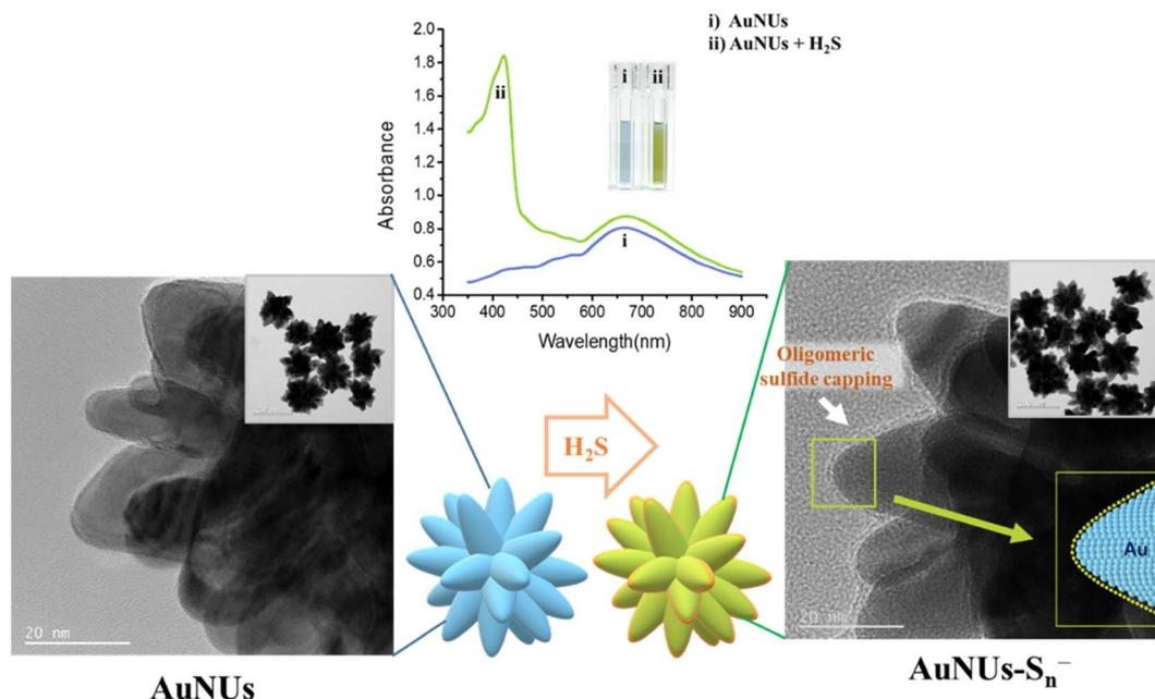
**Scheme 1** Schematic of  $\text{H}_2\text{S}$  detection by gold nanourchins (AuNUs): UV-Vis spectra, a photograph of UV-Vis samples, synthetic morphologies, and HR-TEM images of AuNUs in the absence and the presence of  $\text{H}_2\text{S}$ . HR-TEM image of the oligomeric sulfide capping on the surface of AuNUs in the presence of  $\text{H}_2\text{S}$  ( $150 \mu\text{M}$ ) was zoomed and drawn schematically.
