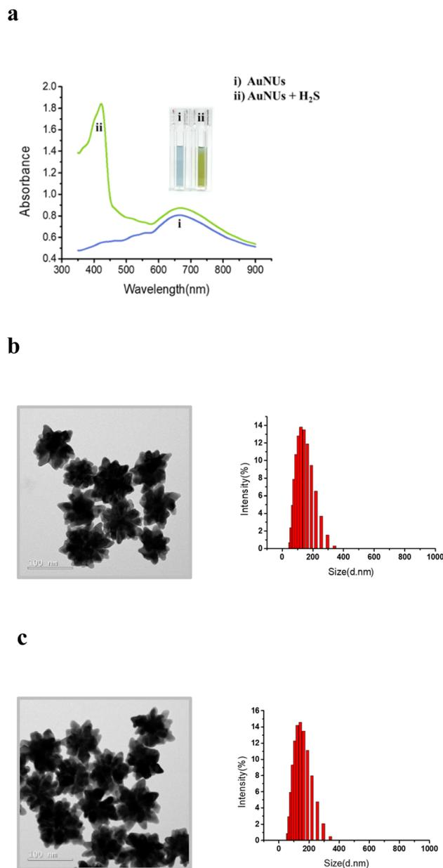
Fig. 1 (a) UV-Vis spectra of AuNUs (sky blue) and AuNUs-H<sub>2</sub>S (light green). (b) HR-TEM image, and the corresponding particle-size distribution ( $d = 115.4$  nm) of AuNUs. (c) HR-TEM image, and the corresponding particle-size distribution ( $d = 122.1$  nm) of AuNUs-H<sub>2</sub>S at pH 4.0 and 25 °C in 20 mM NaCl.
