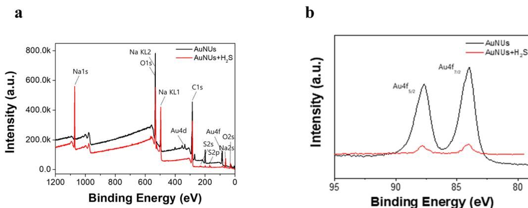
**Fig. 2** (a) Wide-scan XPS spectra of AuNUs (black) and AuNUs- $\text{H}_2\text{S}$  (red). (b) XPS Au4f spectra of AuNUs (black) and AuNUs- $\text{H}_2\text{S}$  (red) at pH 4.0 and 25 °C in 20 mM NaCl.
