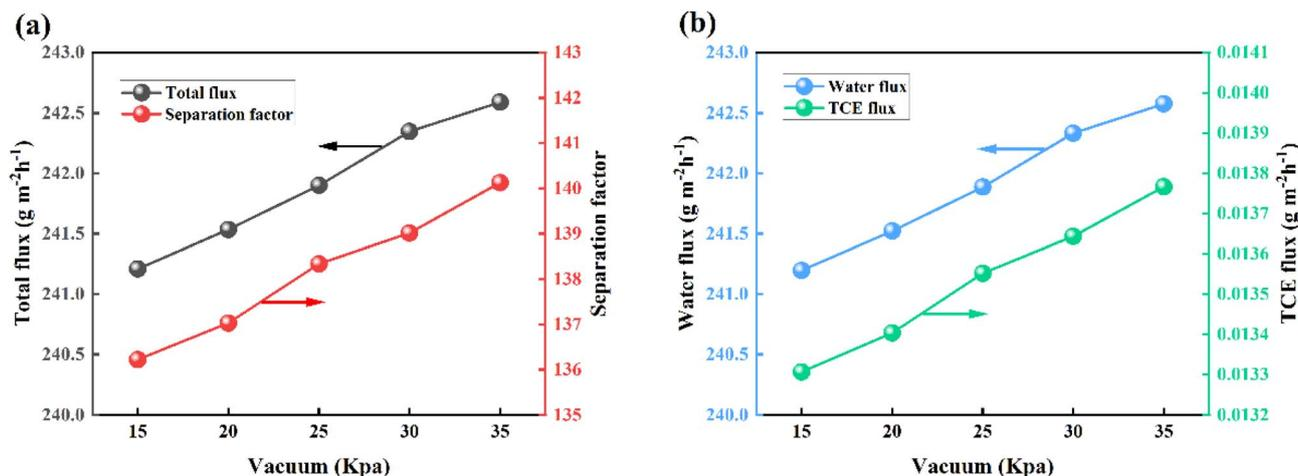
Fig. 17 Effect of permeate-side on PV performance of TMDS@silicalite-1/PDMS membranes with 40 wt% loading for  $3 \times 10^{-7}$  wt% TCE solution. (a) Effects on total flux and separation factor, (b) effect on water flux and TCE flux.
