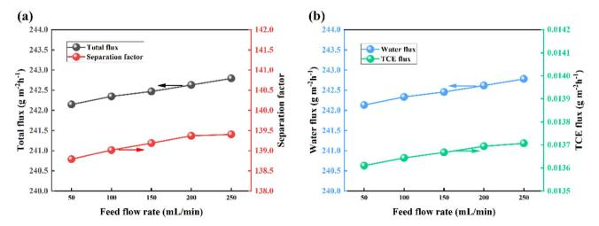
Fig. 16 Effect of feed flow rate on PV performance of TMDS@silicalite-1/PDMS membranes with 40 wt% loading for  $3 \times 10^{-7}$  wt% TCE solution. (a) Effects on total flux and separation factor, (b) effect on water flux and TCE flux.
