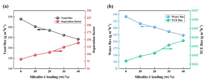
Fig. 13 PV performance of TMDS@silicalite-1/PDMS membranes with different particle loading amounts. (a) Effects on total flux and separation factor, (b) effect on water flux and TCE flux.
