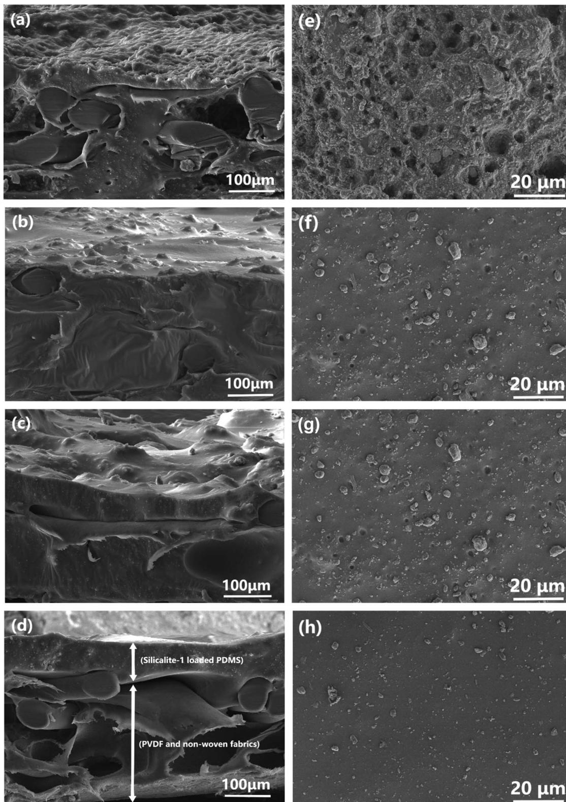
**Fig. 8** Cross-section images of the MMMs doped with 20 wt% (a) unmodified silicalite-1, (b) APTMS@silicalite-1, (c) TMCS@silicalite-1 and (d) TMDS@silicalite-1 particles; surface images of the MMMs doped with 20 wt% (e) unmodified silicalite-1, (f) APTMS@silicalite-1, (g) TMCS@silicalite-1 and (h) TMDS@silicalite-1 particles.
