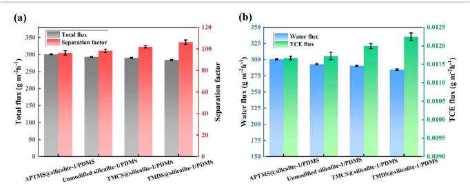
Fig. 10 PV performances of the MMMs doped with APTMS@silicalite-1, unmodified silicalite-1, TMCS@silicalite-1, and TMDS@silicalite-1 particles in a  $3 \times 10^{-7}$  wt% TCE solution at 30 °C
