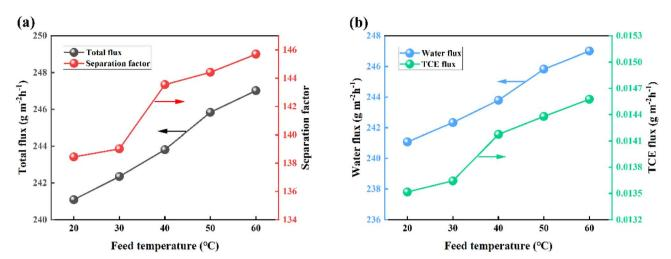
Fig. 15 Effect of feed temperature on PV performance of TMDS@silicalite-1/PDMS membranes with 40 wt% loading for  $3 \times 10^{-7}$  wt% TCE solution. (a) Effects on total flux and separation factor, (b) effect on water flux and TCE flux.
