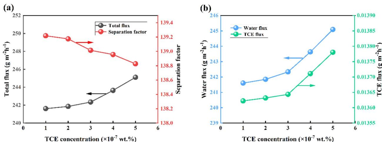
Fig. 14 Effect of feed concentration on PV performance of TMDS@silicalite-1/PDMS membranes with 40 wt% loading for  $3 \times 10^{-7}$  wt% TCE solution. (a) Effects on total flux and separation factor, (b) effect on water flux and TCE flux.
