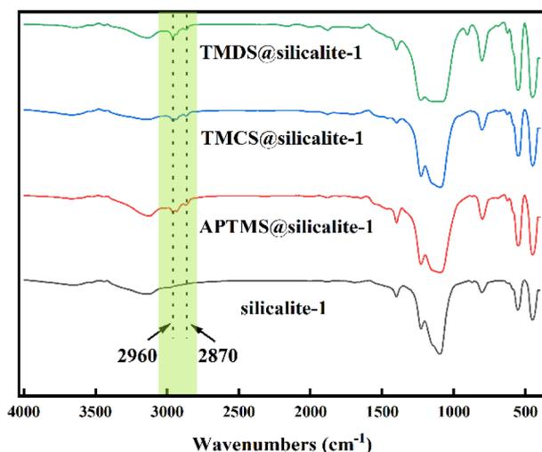
Fig. 5 FTIR spectra of unmodified silicalite-1, APTMS@silicalite-1, TMCS@silicalite-1, and TMDS@silicalite-1.
