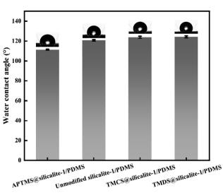
Fig. 9 Water contact angles of the MMMs doped with 20 wt% APTMS@silicalite-1, unmodified silicalite-1, TMCS@silicalite-1 and TMDS@silicalite-1 particles.
