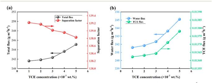
Fig. 14 Effect of feed concentration on PV performance of TMDS@silicalite-1/PDMS membranes with 40 wt% loading for  $3 \times 10^{-7}$  wt% TCE solution. (a) Effects on total flux and separation factor, (b) effect on water flux and TCE flux.
