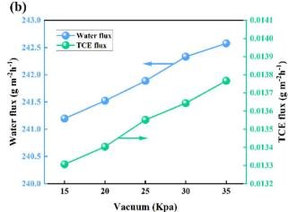
Fig. 17 Effect of permeate-side on PV performance of TMDS@silicalite-1/PDMS membranes with 40 wt% loading for  $3 \times 10^{-7}$  wt% TCE solution. (a) Effects on total flux and separation factor, (b) effect on water flux and TCE flux
