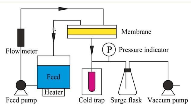
Fig. 3 Schematic diagram of pervaporation apparatus.
