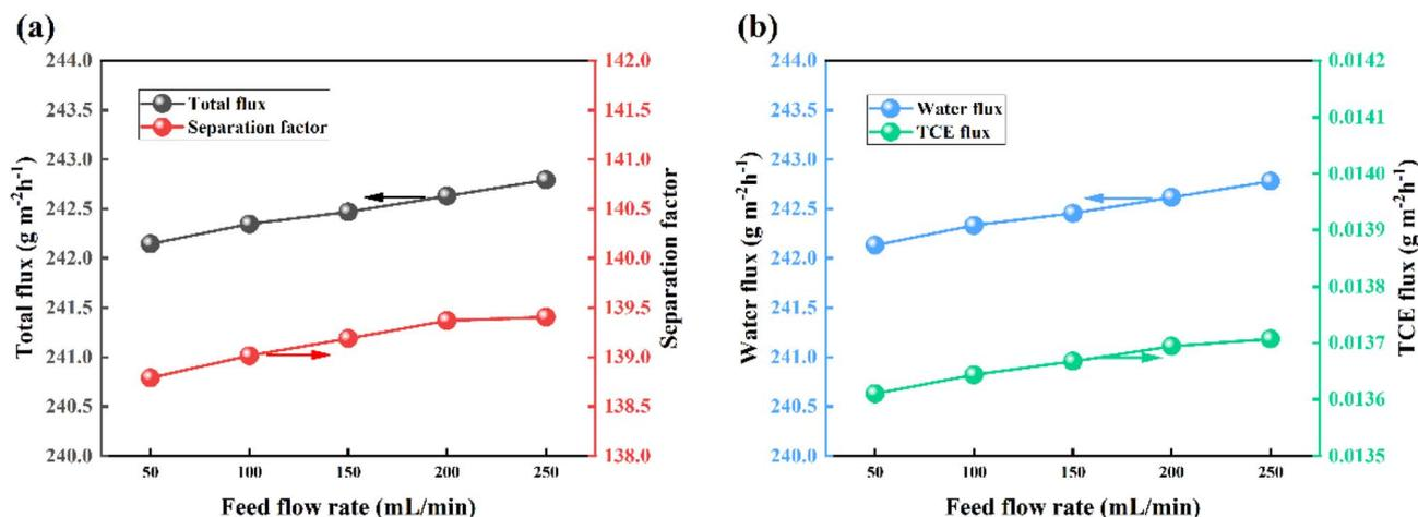
Fig. 16 Effect of feed flow rate on PV performance of TMDS@silicalite-1/PDMS membranes with 40 wt% loading for  $3 \times 10^{-7}$  wt% TCE solution. (a) Effects on total flux and separation factor, (b) effect on water flux and TCE flux.
