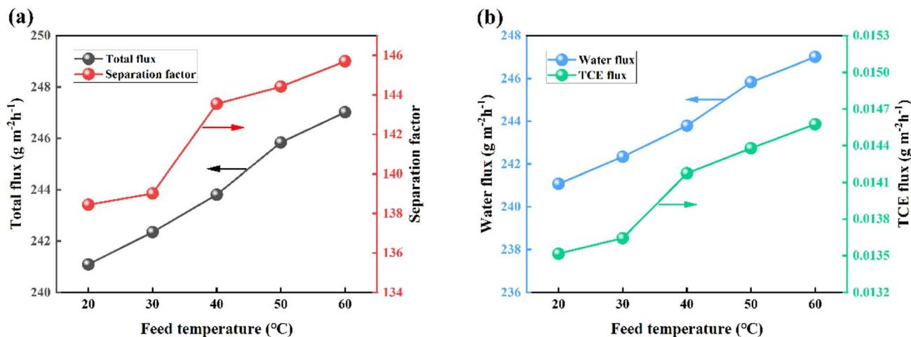
Fig. 15 Effect of feed temperature on PV performance of TMDS@silicalite-1/PDMS membranes with 40 wt% loading for  $3 \times 10^{-7}$  wt% TCE solution. (a) Effects on total flux and separation factor, (b) effect on water flux and TCE flux.
