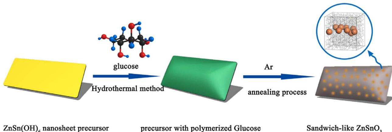
Fig. 19 Schematic illustration depicting the synthesis of sandwich-like ZnSnO<sub>3</sub>@C.<sup>194</sup>
