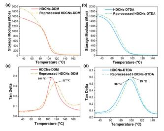
Fig. 4 Storage modulus versus temperature curves of original and reprocessed HDCNs-DDM (a) and HDCNs-DTDA (b). Tan  $\delta$  versus temperature curves of original and reprocessed HDCNs-DDM (c) and HDCNs-DTDA (d)
