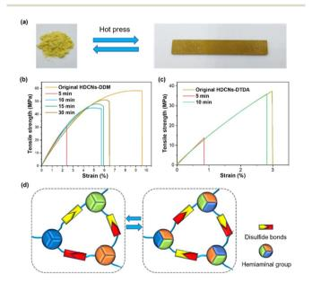
Fig. 3 Photographs of both HDCNs-DTDA before and after reprocessing treatment (a); representative tensile strength-strain curves of original and reprocessed HDCNs-DDM (b) and HDCNs-DTDA (c) with different reprocessing times. Mechanism of reversible network rearrangement for HDCNs-DTDA (d).
