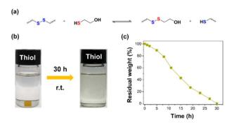
Fig. 5 Thiol-disulfide bond exchange reaction between HDCNs-DTDA and 2-mercaptoethanol (a); chemical degradation of HDCN-DTDA in the 2-mercaptoethanol/DMF solution. (b) Percentage of residual weight of HDCNs-DTDA as a function of time in the 2-mercaptoethanol/DMF solution (c).
