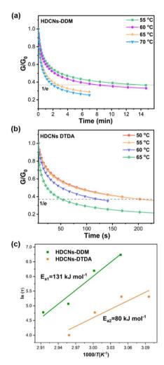
Fig. 2 Stress relaxation of HDCNs-DDM (a) and HDCNs-DTDA (b) at different temperatures. Arrhenius fitted line of the characteristic relaxation time  $\tau$  versus 1000/T for HDCNs (c).
