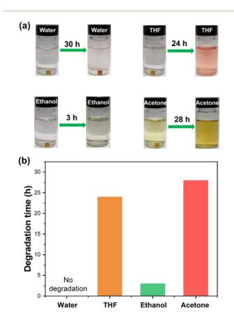
**Fig. 6** Chemical degradation (a) and degradation time (b) of HDCNs-DTDA in HCl solutions containing different organic solvents.
