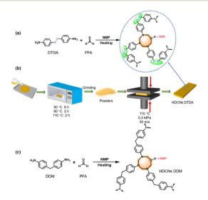
Scheme 1 (a) Synthetic route of HDCNs DTDA from DTDA and PFA. (b) Preparation procedures of HDCNs DTDA. (c) Synthetic route of HDCNs from DDM and PFA.
