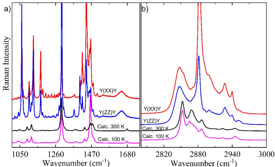
Fig. 7 Room-temperature experimental polarized Raman in the  $y(xx)y$  (red spectrum) and  $y(zz)y$  (blue spectrum) scattering geometries and calculated (scaled) spectra of AA in  $B_m$  form at 300 K (black spectrum) and 100 K (pink spectrum) for regions: (a) 1100–1690  $\text{cm}^{-1}$  and (b) 2780–3000  $\text{cm}^{-1}$ .
