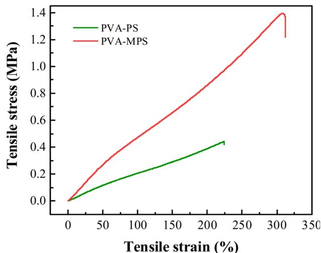
Fig. 3 Strain-stress curves PVA-PS and PVA-MPS hydrogels.
