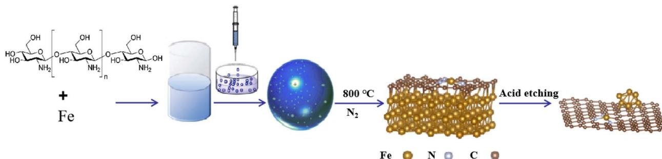
Scheme 1 Preparation process of the FeA-NC catalyst.
