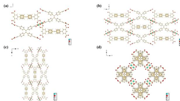
Fig. 1 Perspective view of the crystal structure of Cu-MOF (a) complex structure of the Cu-metal node (b) crystal structure of Cu-MOF along the crystallographic *a*-axis, (c) *b*-axis, and (d) *c*-axis. C, grey; O, red; Zn, blue; H, white.
