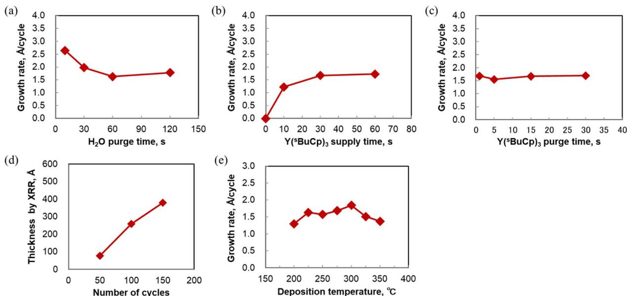
Fig. 5 (a) Growth rate for  $Y_2O_3$  films as function of water purge time at 250 °C. (b) Saturation of  $Y_2O_3$  film growth rate with increasing  $Y(^sBuCp)_3$  supply time at 250 °C. (c)  $Y_2O_3$  film growth rate as function of the  $Y(^sBuCp)_3$  purge time at 250 °C. (d) Film thickness as function of number of ALD cycles at 250 °C. (e) Growth rate for  $Y_2O_3$  films as function of deposition temperature.
