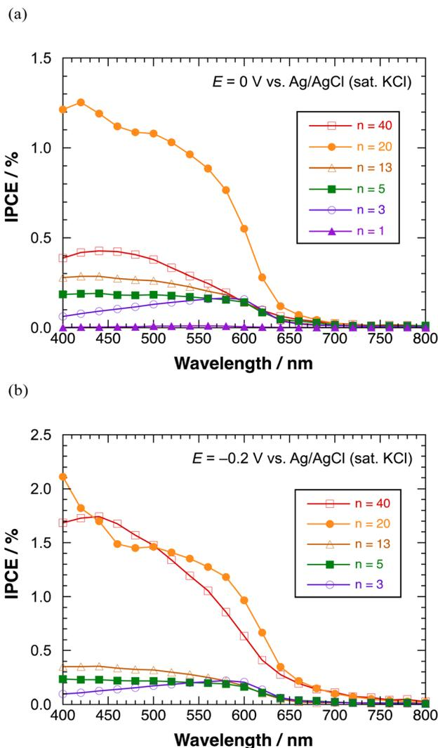
Fig. 8 IPCE profiles of polyBiTh( $n$ )/C<sub>60</sub>PF/PSS/PEI/ITO in the presence of methyl viologen at (a) 0 V, and (b)  $-0.2$  V versus Ag/AgCl (sat. KCl).
