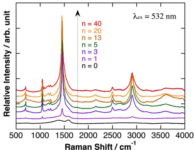
Fig. 4 Relative Raman scattering spectra of polyBiTh(*n*)/C<sub>60</sub>PF/PSS/PEI/ITO, after baseline correction and adjusted for comparison. Relative intensities of Raman signals were not adjusted.
