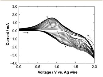
Fig. 2 Cyclic voltammogram of the electrochemical polymerization of polyBiTh on  $C_{60}$ PF/PSS/PEI/ITO during preparation of polyBiTh(20)/  $C_{60}$ PF/PSS/PEI/ITO.
