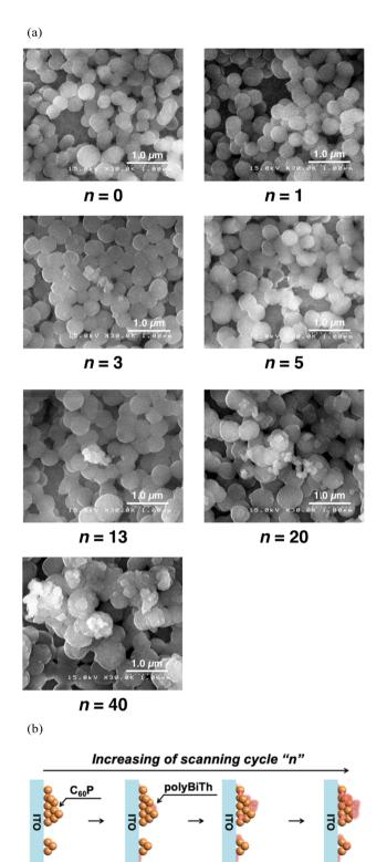
Fig. 5 (a) SEM images of polyBiTh(n)/C<sub>60</sub>PF/PSS/PEI/ITO (n = 0, 1, 3, 5, 13, 20, and 40 cycles), and (b) proposed mechanism of polyBiTh thin-films growing on C<sub>60</sub>PF/PSS/PEI/ITO.
