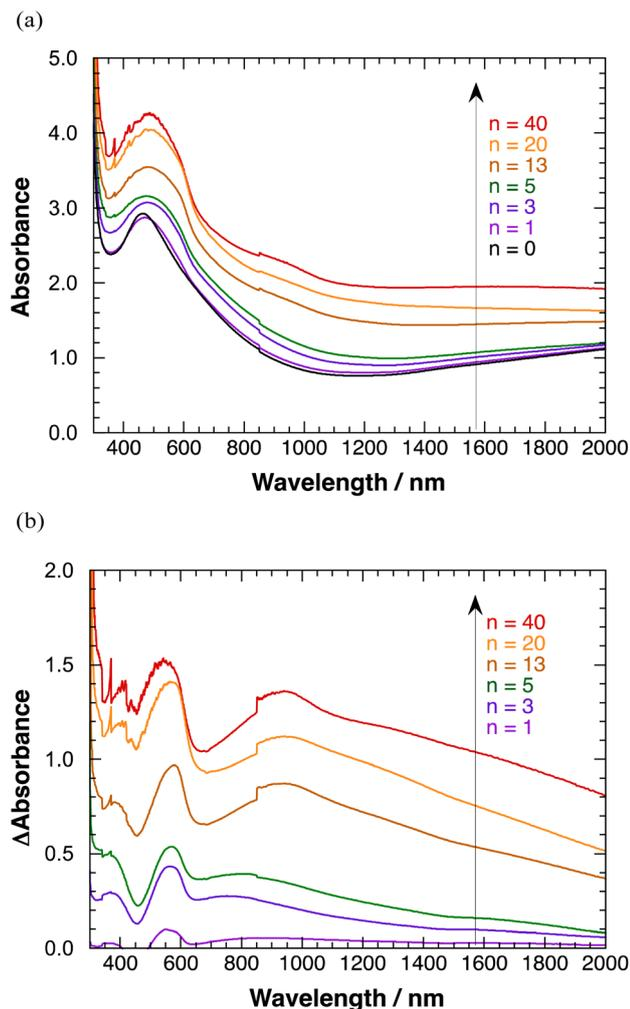
Fig. 6 (a) Transmission absorption spectra of polyBiTh( $n$ )/C<sub>60</sub>PF/PSS/PEI/ITO, and (b) differential transmission absorption spectra of polyBiTh( $n$ )/C<sub>60</sub>PF/PSS/PEI/ITO after subtraction of C<sub>60</sub>PF/PSS/PEI/ITO absorption spectra.
