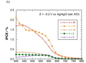
Fig. 8 IPCE profiles of polyBiTh $(n)/C_{60}$ PF/PSS/PEI/ITO in the presence of methyl viologen at (a) 0 V, and (b) -0.2 V versus Ag/AgCl (sat. KCl).
