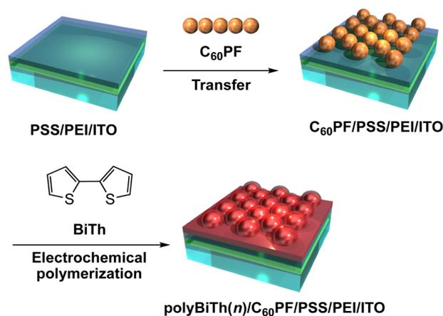
Fig. 1 Fabrication of polybithiophene electrochemically polymerized thin-film modified densely packed C<sub>60</sub>–ethylenediamine adduct microparticles film.
