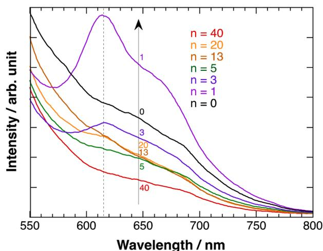
Fig. 7 Fluorescence emission spectra of polyBiTh( $n$ )/C<sub>60</sub>PF/PSS/PEI/ITO,  $\lambda_{\text{ex}} = 450$  nm.
