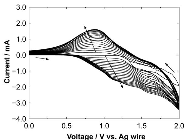
Fig. 2 Cyclic voltammogram of the electrochemical polymerization of polyBiTh on C<sub>60</sub>PF/PSS/PEI/ITO during preparation of polyBiTh(20)/C<sub>60</sub>PF/PSS/PEI/ITO.
