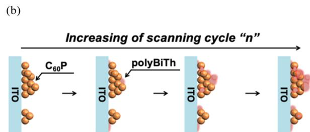
Fig. 5 (a) SEM images of polyBiTh(*n*)/C<sub>60</sub>PF/PSS/PEI/ITO (*n* = 0, 1, 3, 5, 13, 20, and 40 cycles), and (b) proposed mechanism of polyBiTh thin-films growing on C<sub>60</sub>PF/PSS/PEI/ITO.
