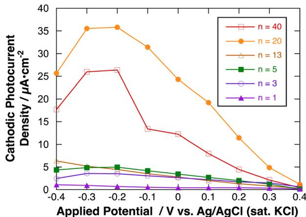
Fig. 9 Applied potential dependence of cathodic photocurrent of polyBiTh(*n*)/C<sub>60</sub>PF/PSS/PEI/ITO.
