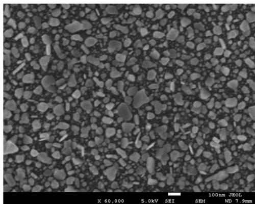
Fig. 7 SEM image of the front of a poly(dopamine acrylamide) (pDOPAm) thin film with electroless-deposited silver. Electroless deposition was performed at 80 °C for 24 h using aqueous AgNO<sub>3</sub>.
