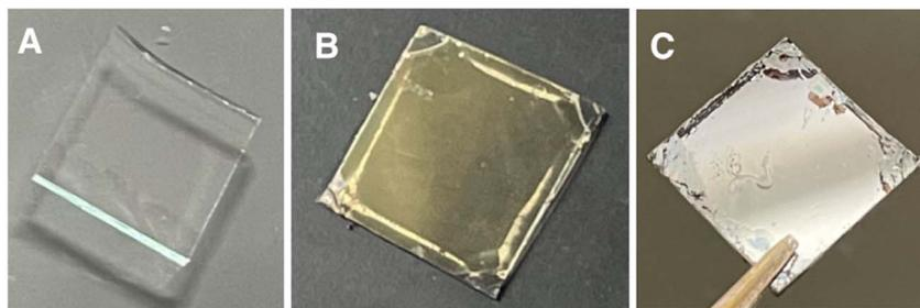
Fig. 4 Images of poly(dopamine acrylamide) (pDOPAm) thin films on glass substrates. Front side of the films after thermal annealing (A) under vacuum and (B) in aqueous  $\text{AgNO}_3$  for 24 h. (C) Back side of the film shown in (B).
