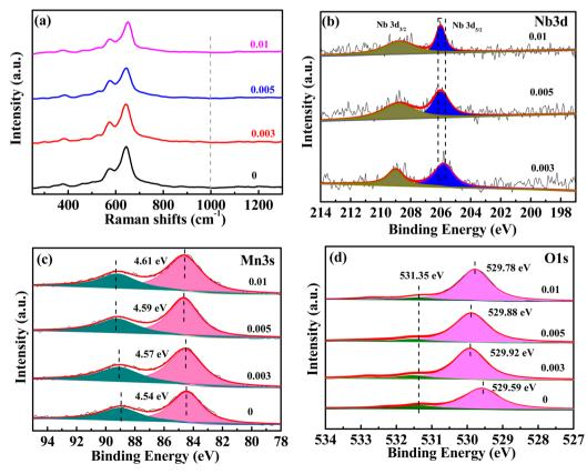
Fig. 2 Raman spectra (a), XPS spectra for Nb 3d (b), Mn 3s (c), and O 1s (d) of MnO<sub>2</sub> with different Nb/Mn molar ratios.
