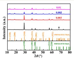
Fig. 1 The XRD patterns of MnO<sub>2</sub> doped with different amounts of Nb.
