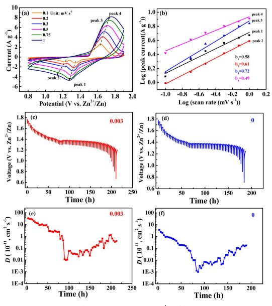
Fig. 6 (a) CV curves at different sweep velocities (0.1, 0.2, 0.3, 0.5, 0.75, and  $1 \,\mathrm{mV} \,\mathrm{s}^{-1}$ ) and (b)  $\log i$  and  $\log v$  plots at specific peak currents; (c and d) GITT profiles at discharge state and (e and f) the corresponding ion diffusion coefficients of the 0.003 sample and undoped MnO<sub>2</sub>.
