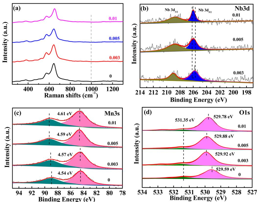
Fig. 2 Raman spectra (a), XPS spectra for Nb 3d (b), Mn 3s (c), and O 1s (d) of MnO<sub>2</sub> with different Nb/Mn molar ratios.
