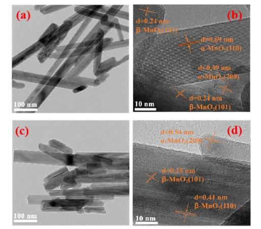
Fig. 3 TEM and HRTEM morphology of samples with Nb/Mn molar ratios of 0 (a and b), and 0.003 (c and d).
