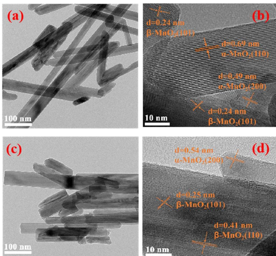
**Fig. 3** TEM and HRTEM morphology of samples with Nb/Mn molar ratios of 0 (a and b), and 0.003 (c and d).
