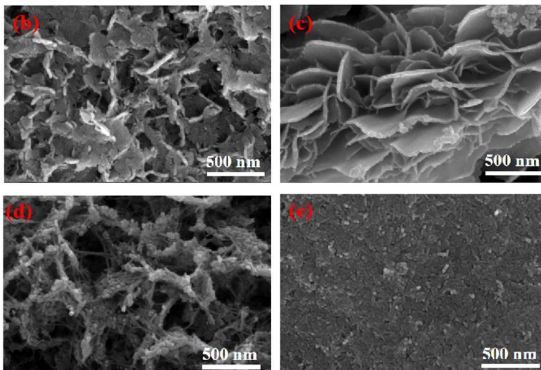
Fig. 5 XRD patterns (a) and SEM morphology of the 0.003 sample recharging 1.9 V after 10 cycles (b), 50 cycles (c), 100 cycles (d), and 200 cycles (e) at 1C.
