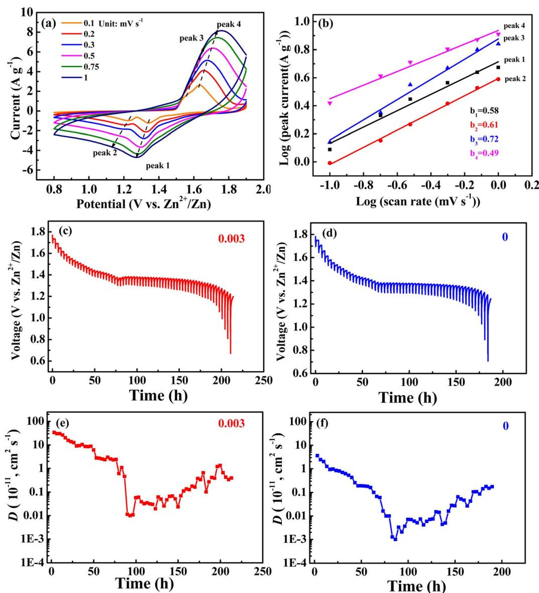
Fig. 6 (a) CV curves at different sweep velocities (0.1, 0.2, 0.3, 0.5, 0.75, and 1  $\text{mV s}^{-1}$ ) and (b)  $\log i$  and  $\log v$  plots at specific peak currents; (c and d) GITT profiles at discharge state and (e and f) the corresponding ion diffusion coefficients of the 0.003 sample and undoped  $\text{MnO}_2$ .
