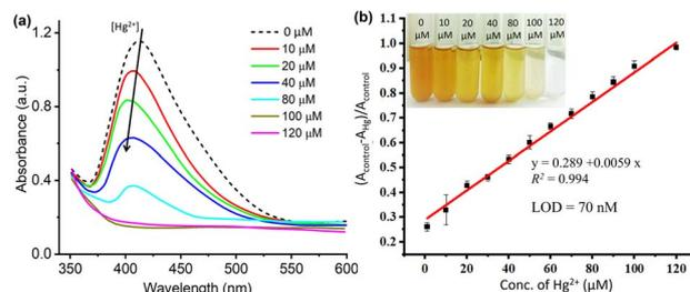
**Fig. 6** (a) UV-vis spectra of ED-AgNPs solution after the addition of different concentrations of mercury(II) ions. (b) Corresponding linear plot of the relative absorbance intensity difference at peak maxima versus  $\text{Hg}^{2+}$  concentration. Error bars represent the standard deviation of three repeated measurements. Inset: photograph of respective solutions at different concentrations.
