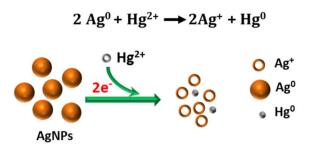
Fig. 7 Illustration of the proposed redox reaction mechanism underlying the colorimetric sensing of Hq<sup>2+</sup> using ED-AgNPs.
