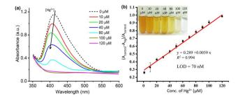
**Fig. 6** (a) UV-vis spectra of ED-AgNPs solution after the addition of different concentrations of mercury(II) ions. (b) Corresponding linear plot of the relative absorbance intensity difference at peak maxima *versus* Hg<sup>2+</sup> concentration. Error bars represent the standard deviation of three repeated measurements. Inset: photograph of respective solutions at different concentrations.
