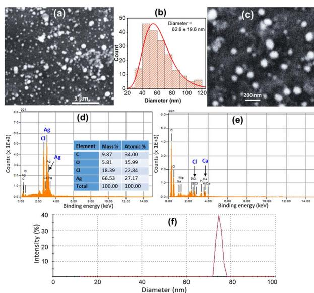
Fig. 4 (a and c) SEM images of ED-AgNPs with different magnifications. (b) Size distribution histogram with the longnorm curve; the average size  $\pm$  standard deviation is given. EDX spectrum of (d) ED-AgNPs and (e) ED extract; inset shows the elemental analysis from EDX. (f) DLS data of as-prepared ED-AgNPs.
