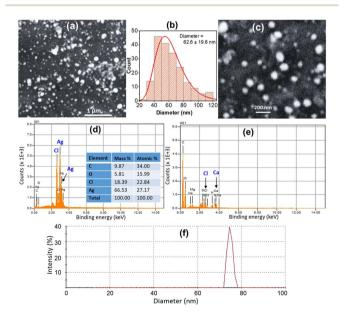
Fig. 4 (a and c) SEM images of ED-AgNPs with different magnifications. (b) Size distribution histogram with the longnorm curve; the average size  $\pm$  standard deviation is given. EDX spectrum of (d) ED-AgNPs and (e) ED extract; inset shows the elemental analysis from EDX. (f) DLS data of as-prepared ED-AgNPs.
