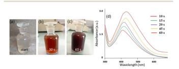
Fig. 2 Photographs of 1 mM  $AgNO_3$  + ED extract mixture after exposure to sunlight for (a) 0 s (start), (b) 30 s, and (c) 60 s showing color changes with time. (d) UV-vis spectra of ED-AgNPs suspension after different reaction times.
