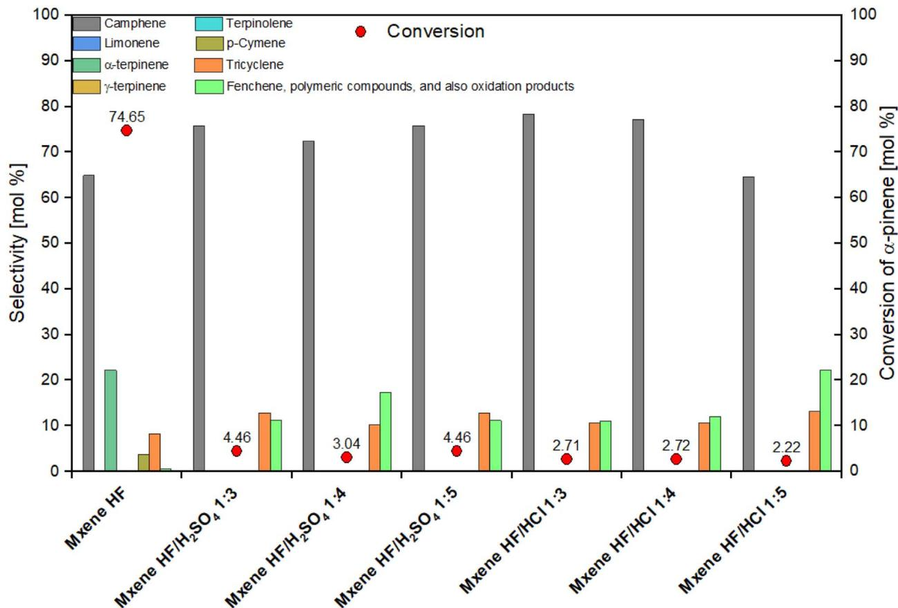
Fig. 7 Results of the catalytic tests for the isomerization of  $\alpha$ -pinene for MXene HF, MXene HF/H<sub>2</sub>SO<sub>4</sub> X : Y, and MXene HF/HCl X : Y.
