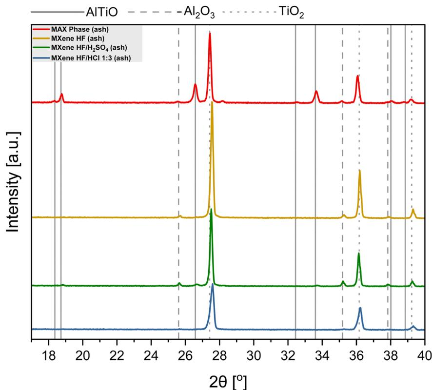
Fig. 5 XRD patterns of MAX phase, MXene HF/H<sub>2</sub>SO<sub>4</sub> 1 : 3 and MXenes HF/HCl 1 : 3 after TGA.
