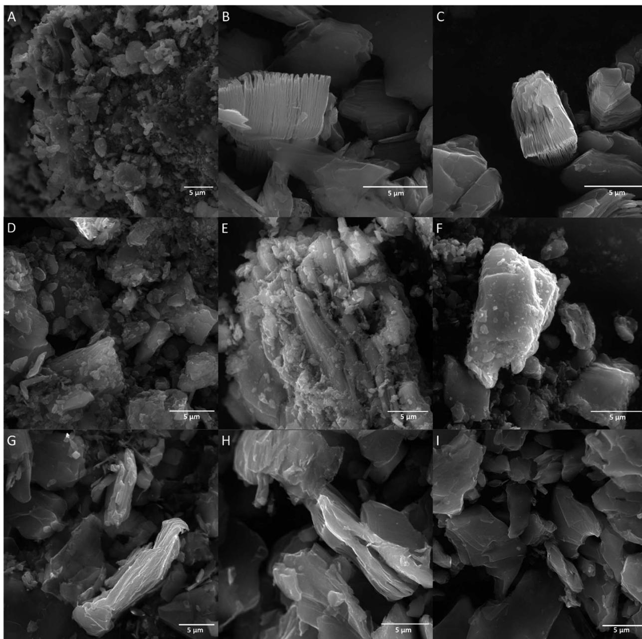
Fig. 1 SEM images of MAX phase (A), MXene HF (B and C), MXene  $\text{HF}/\text{H}_2\text{SO}_4$  1 : 3 (D), MXene  $\text{HF}/\text{H}_2\text{SO}_4$  1 : 4 (E), MXene  $\text{HF}/\text{H}_2\text{SO}_4$  1 : 5 (F), MXene  $\text{HF}/\text{HCl}$  1 : 3 (G), MXene  $\text{HF}/\text{HCl}$  1 : 4 (H), MXene  $\text{HF}/\text{HCl}$  1 : 5 (I).
