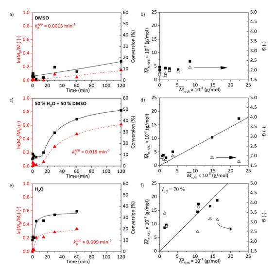
Fig. 1 Kinetic plots and the evolution of molecular weight and dispersity for SET-RDRP of NAGA in degassed DMSO (a and b), DMSO/H<sub>2</sub>O (1/1, v/v, c and d) and H<sub>2</sub>O (e and f) at 45 °C under the conditions  $[M]_0: [L]_0: [L]_0: [Cu^{ll}]_0 = 500:1:2:1$  and catalysis of a copper wire (6 cm). Data were fitted with a 5PL fit. The  $k_p^{\text{op}}$  was calculated as the maximum of the first derivative.
