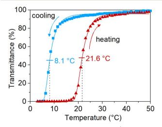
Fig. 5 Turbidimetry curve of PNAGA (18 700 g mol $^{-1}$ , D=3.1, from the kinetic study in Fig. 1e, f) in deionized water. The data were fitted with 5PL fit and the cloud points were determined from the inflection points.
