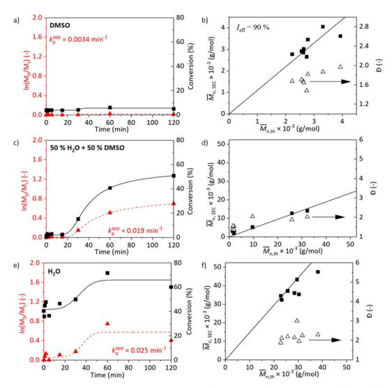
Fig. 2 Kinetic plots with the evolution of molecular weight and dispersity for SET-RDRP of NAGAm in degassed DMSO (a and b), DMSO/H<sub>2</sub>O (1/1, v/v, c and d) and H<sub>2</sub>O (e and f) at 25 °C under the conditions  $[M]_0 : [L]_0 : [Cu^{ll}]_0 = 500 : 1 : 2 : 1$  and catalysis of a copper wire (6 cm). Data were fitted with a 5PL fit. The  $k_p^{app}$  was calculated as the maximum of the first derivative.
