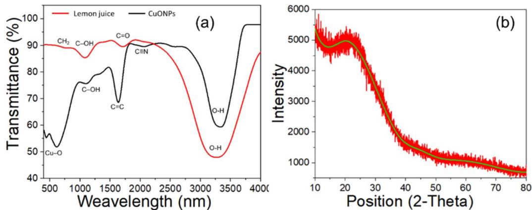
Fig. 3 FTIR spectra and XRD data obtained from lemon juice and green synthesized CuONPs using lemon juice as reducing agent.
