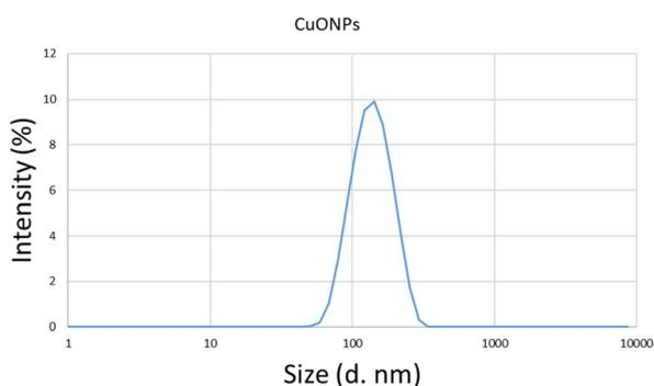
Fig. 5 The hydrodynamic size distribution spectrum of CuONPs using DLS.
