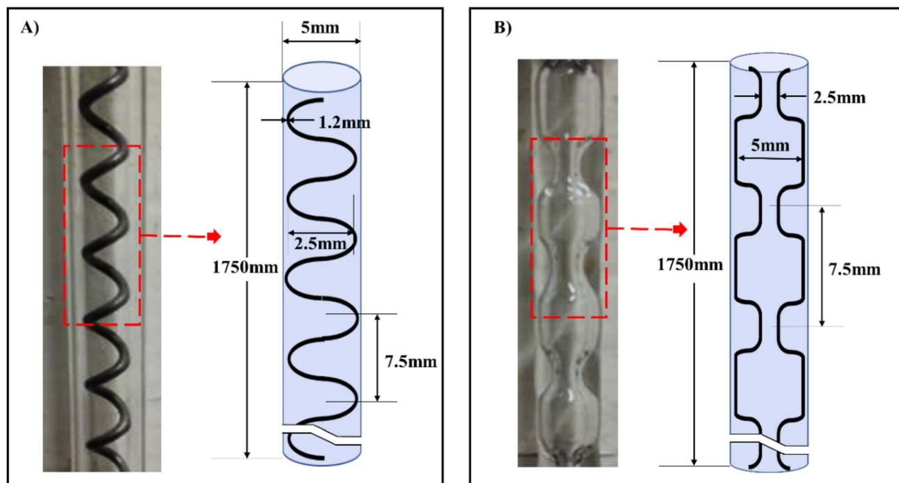
Fig. 10 Meso-OBRs designs configuration and schematics of the conventional, (A) helical baffles (B) integral baffles.<sup>5</sup>
