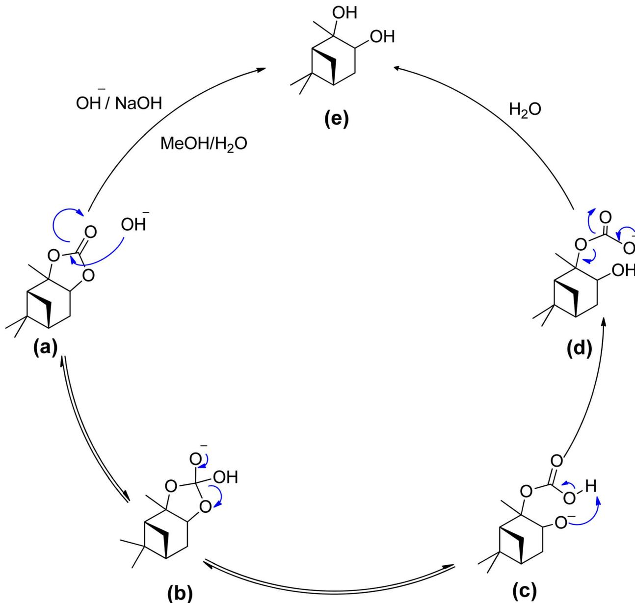
Scheme 18 Proposed reaction mechanism - a bimolecular collision of solvated hydroxide ion with the alky esters carbonyl carbon.<sup>88</sup>
