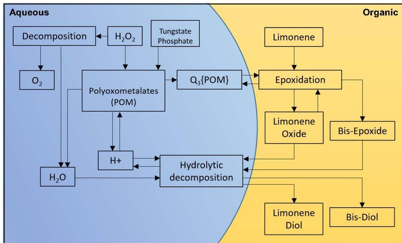
Fig. 5 Overall reaction scheme for the epoxidation of (*R*)-(+)-limonene, the formation of oxidative species, the decomposition of  $\text{H}_2\text{O}_2$  and the hydrolytic decomposition of the epoxides. Each reaction is visualized in the schematic diagram (an aqueous phase is shown in blue, while an organic phase is shown in gold).
