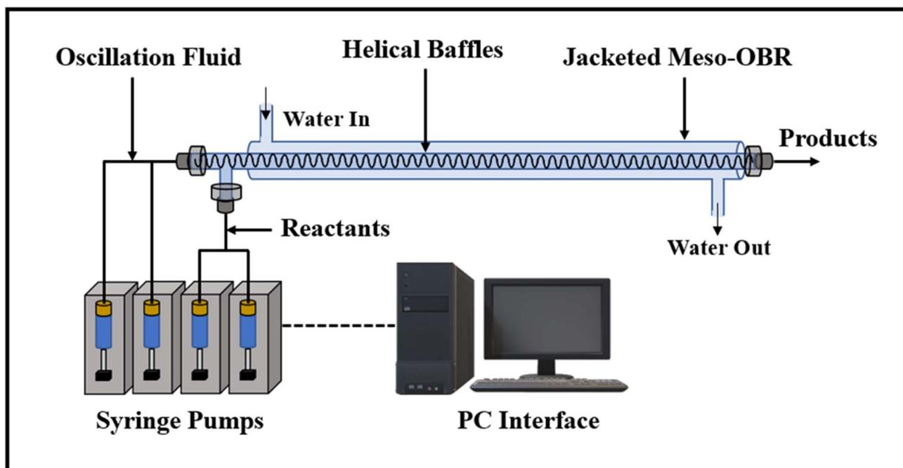
Fig. 12 The helically baffled meso-OBR is used for the flow epoxidation of terpenes with  $\text{H}_2\text{O}_2$ .<sup>5</sup>
