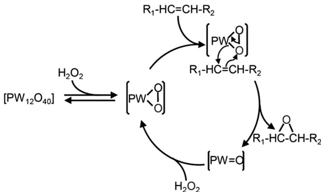
Scheme 22 Reaction mechanism of alkene epoxidation using Venturello anion as the catalyst.<sup>114</sup>
