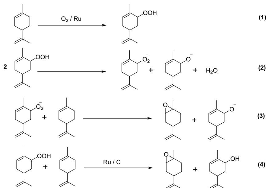
Scheme 10 Proposed chemical route for solvent- and initiator-free aerobic limonene oxidation.<sup>31</sup>
