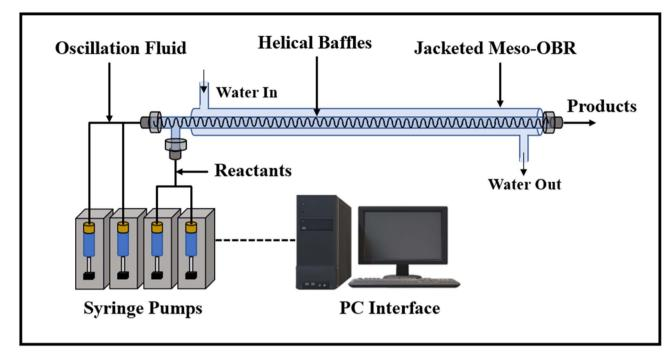
Fig. 12 The helically baffled meso-OBR is used for the flow epoxidation of terpenes with H<sub>2</sub>O<sub>2</sub>.<sup>5</sup>
