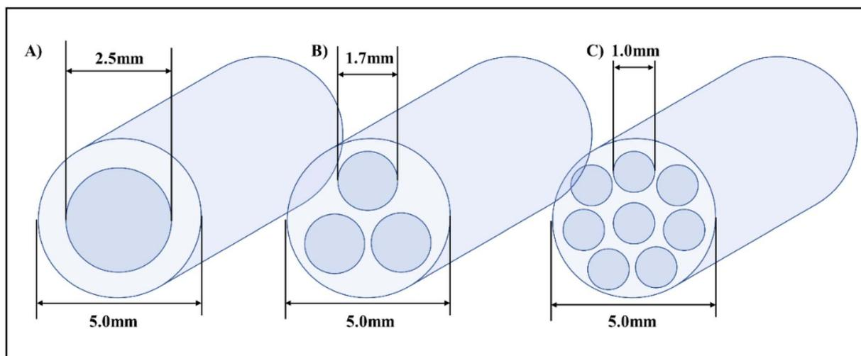
Fig. 11 Orifice meso-OBR design schematics and configurations for 3D printing, (A) single orifice (B) tri-orifice (C) Multi-orifice.<sup>5</sup>
