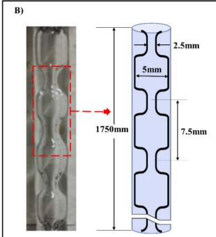
Meso-OBRs designs configuration and schematics of the conventional, (A) helical baffles (B) integral baffles.<sup>5</sup>
