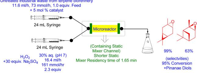
Fig. 14 Catalytic flow epoxidation of Untreated Industrial waste from biorefinery using Venturello Phase Transfer Catalyst (VPTC) (Reproduced from ref. 166)
