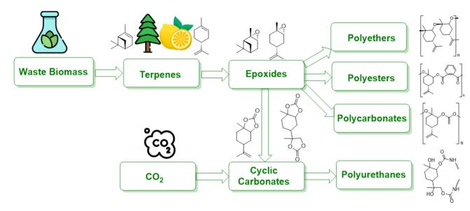
Fig. 1 Multiple routes to polymerize epoxides derived from biomass.
