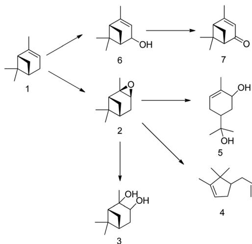
**Scheme 16** Product of  $\alpha$ -pinene epoxidation with hydrogen peroxide ( $\text{H}_2\text{O}_2$ ) as an oxidant in the presence of a tungsten-based catalyst; (1)  $\alpha$ -pinene, (2)  $\alpha$ -pinene oxide, (3) pinanediol, (4) campholenic aldehyde, (5) sobrerol, (6) verbenol and (7) verbenone.
