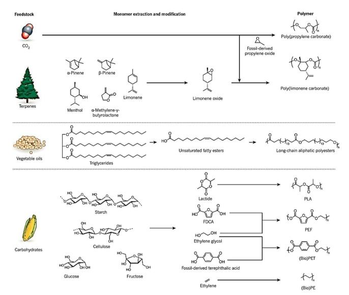
Fig. 2 Bio-based alternatives to petrochemicals for the manufacturing of polymers.<sup>1</sup>
