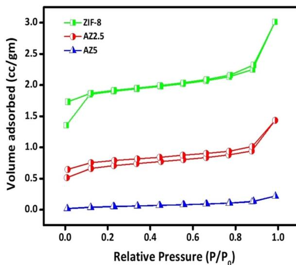
Fig. 8 Nitrogen sorption isotherms of the prepared catalysts.
