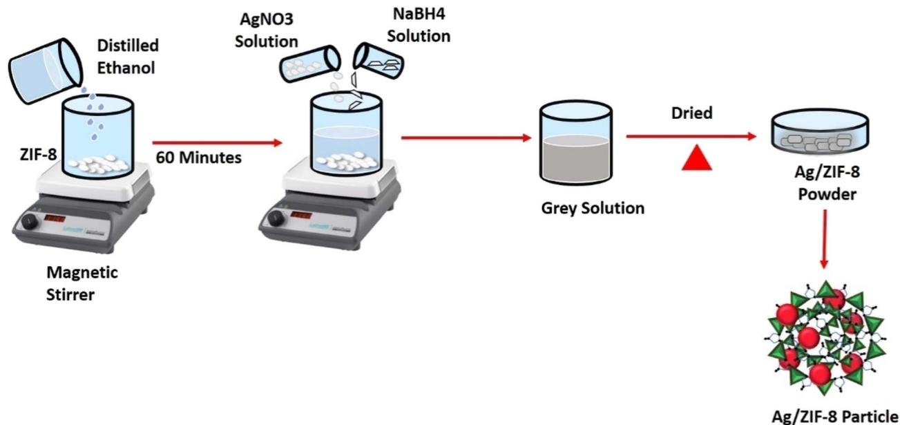
Fig. 2 Schematic diagram of synthesis of Ag/ZIF-8 (reduced).
