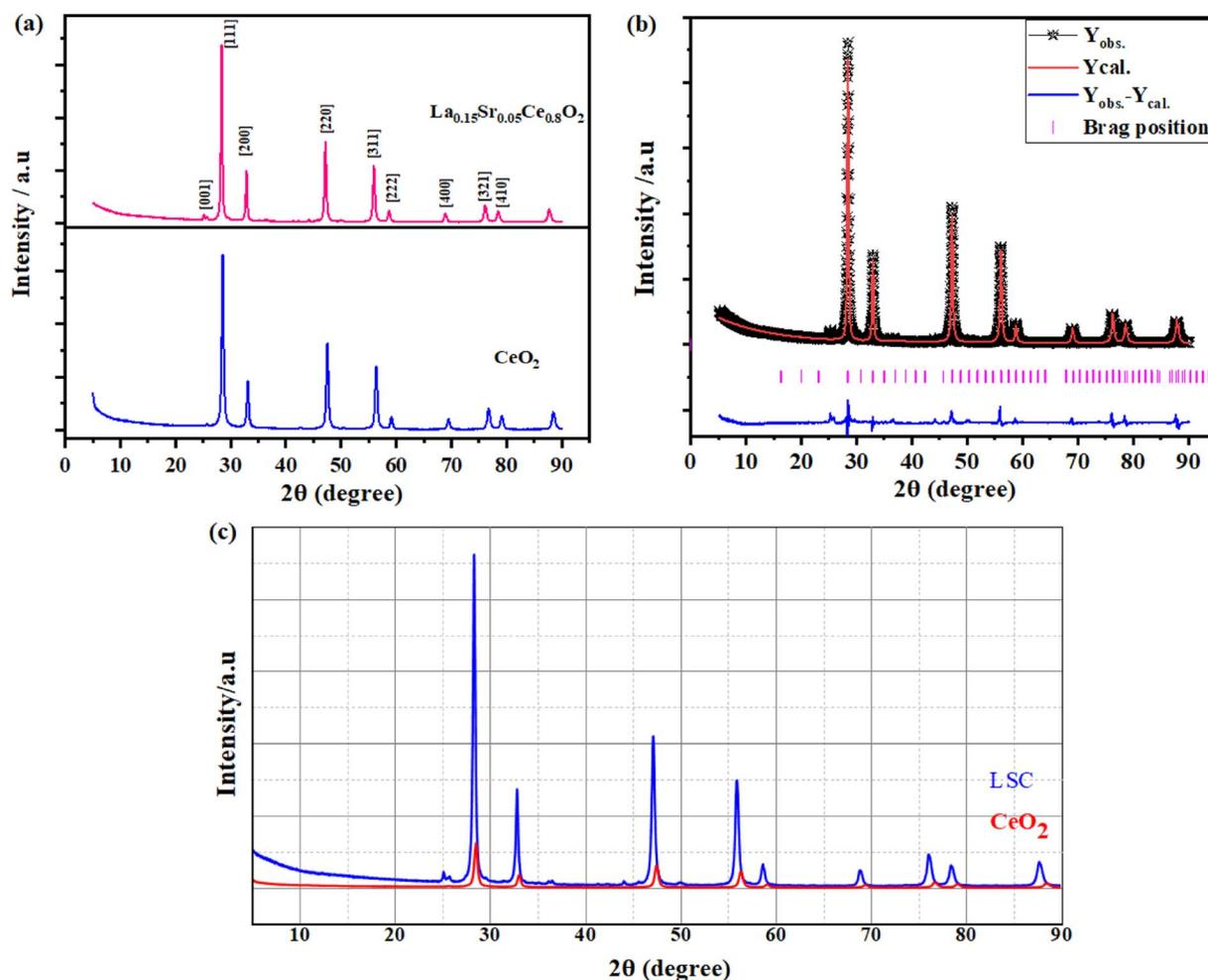
Fig. 1 (a and b) Comparison of the measured XRD data of pristine  $\text{CeO}_2$  and La, Sr-doped  $\text{CeO}_2$ , (b) Rietveld refinement using the Prof-Suit software for the individual La, Sr-doped  $\text{CeO}_2$  and (c) comparison of the peak shifting of the doped and undoped  $\text{CeO}_2$  XRD patterns, respectively.
