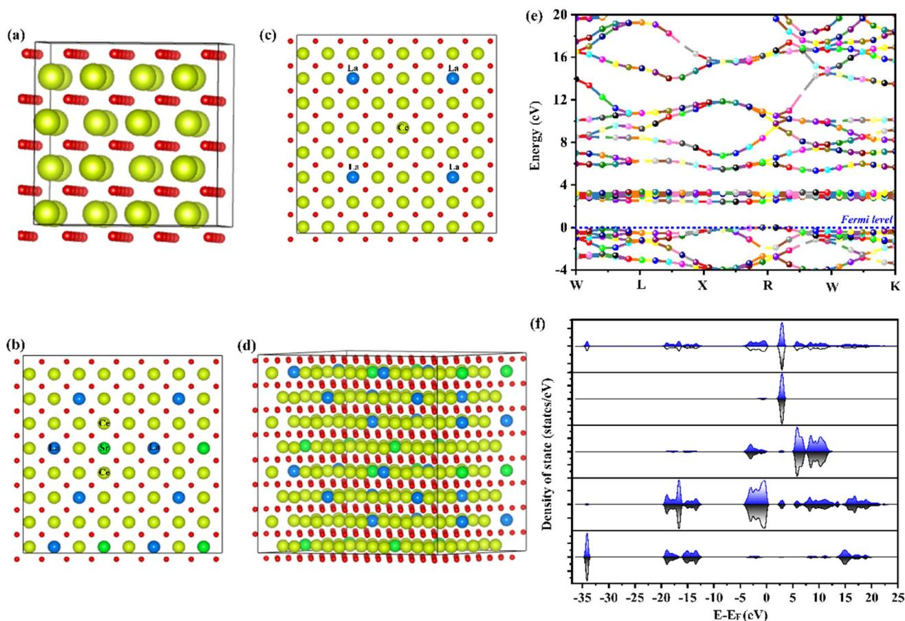
Fig. 8 (a–d) Optimized structure of pure CeO<sub>2</sub>, La-doped CeO<sub>2</sub>, and La and Sr-doped CeO<sub>2</sub>, respectively. (e and f) Calculated energy band structure and DOS results performed for the different orbitals of each species, such as s, p, f, and total DOS for the LSC structure.
