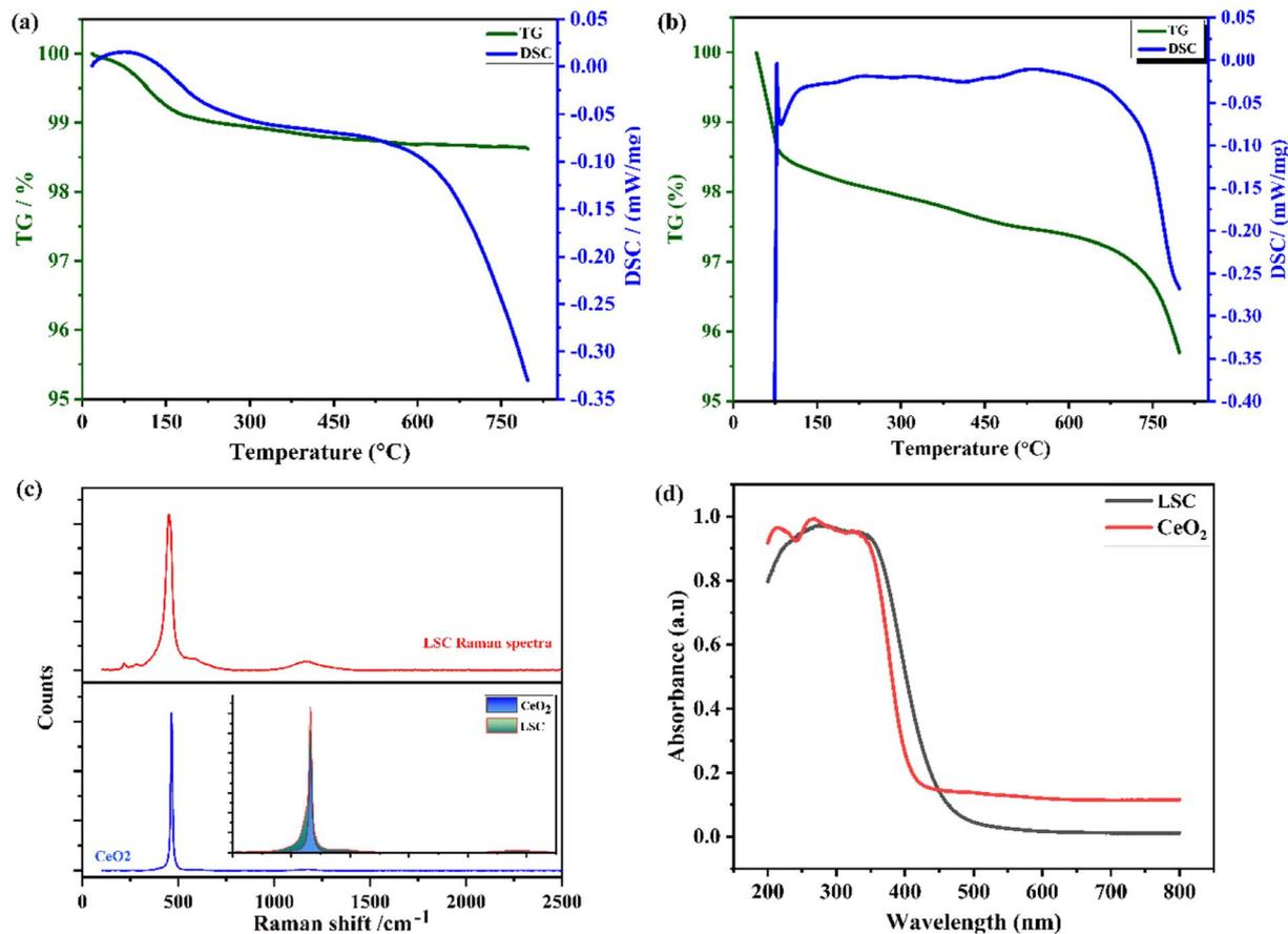
Fig. 5 (a and b) Thermogravimetric and differential scanning calorimetry analysis (TGA/DSC) for evaluating the thermal properties of  $\text{CeO}_2$  and LSC, respectively. (c and d) Raman and UV-visible absorbance and spectra of the  $\text{CeO}_2$  and LSC electrolytes, respectively.
