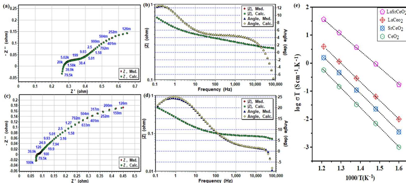
Fig. 7 (a and b) Nyquist and Bode plots of the impedance spectra measured in  $\text{H}_2/\text{air}$  at 550 °C with the corresponding fitting data for fuel cells with  $\text{CeO}_2$  electrolyte. (c and d) Nyquist and Bode plots of the impedance spectra measured in  $\text{H}_2/\text{air}$  at 550 °C with the corresponding fitting data for fuel cells with LSC electrolyte. (e) Comparison of the ionic conductivity of LSC with other developed electrolytes.
