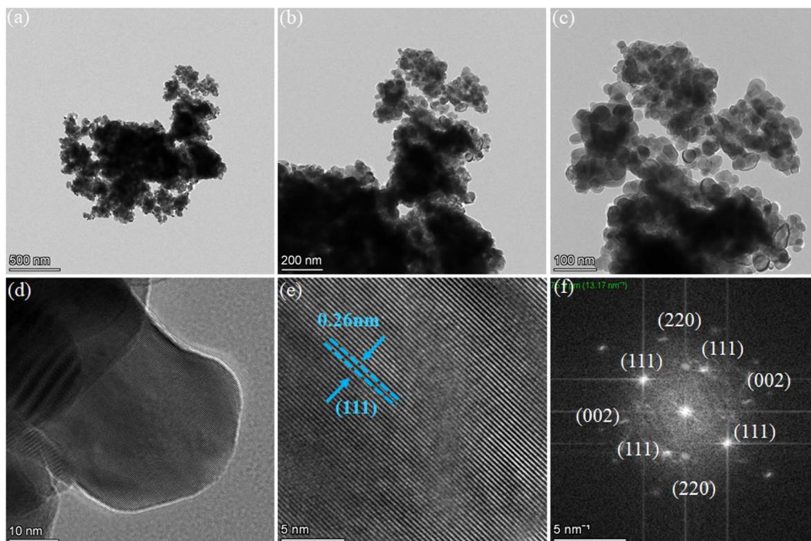
Fig. 2 (a–f) HR-TEM images of  $\text{La}_{0.15}\text{Sr}_{0.05}\text{Ce}_{0.8}\text{O}_{2-\delta}$ : (a–c) morphology display of LSC at different scales: 500, 200, and 100 nm, (d and e), crystal planes of the  $\text{La}_{0.15}\text{Sr}_{0.05}\text{Ce}_{0.8}\text{O}_{2-\delta}$  sample, where the (111) *d*-spacing plane can be observed, and (f) selected area electron diffraction pattern of  $\text{La}_{0.15}\text{Sr}_{0.05}\text{Ce}_{0.8}\text{O}_{2-\delta}$ , respectively.
