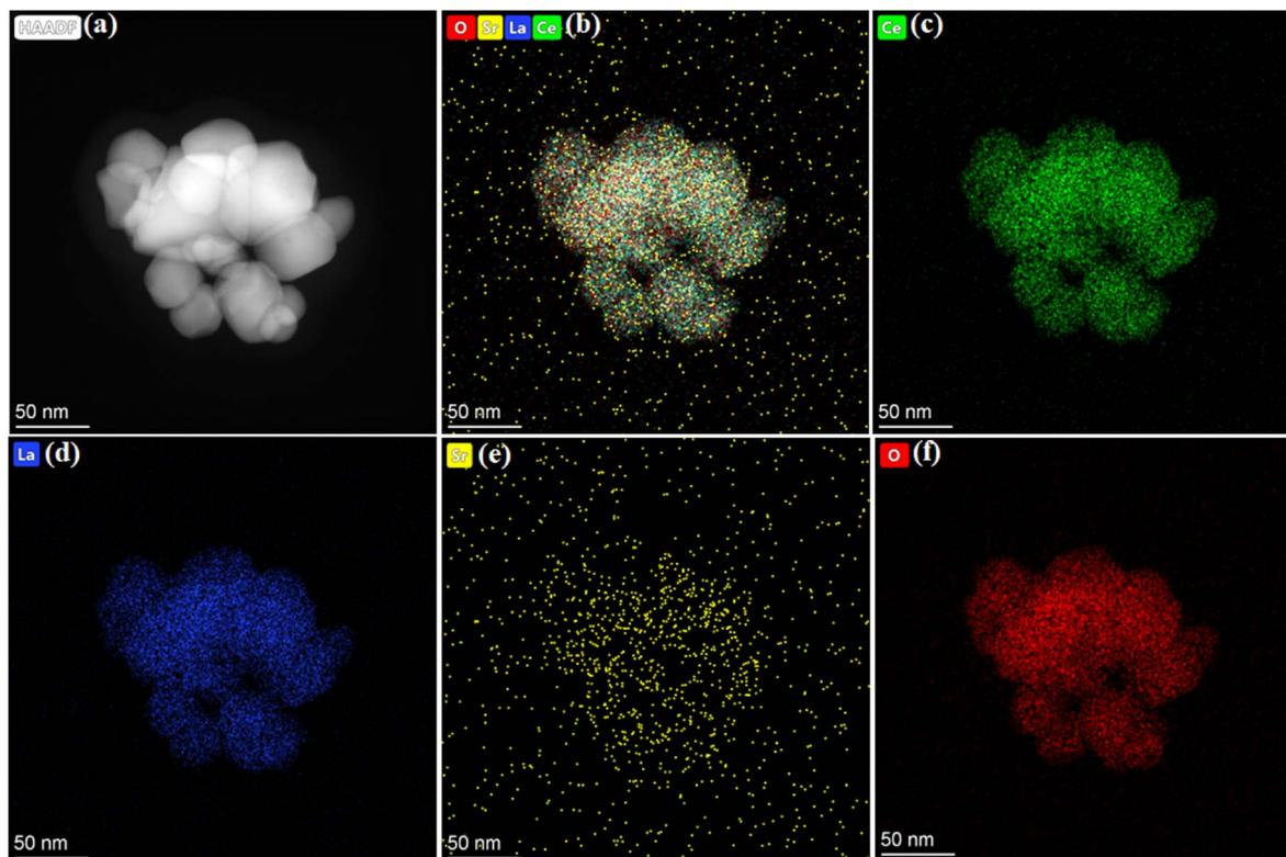
Fig. 3 (a) High annular dark-field image of  $\text{La}_{0.15}\text{Sr}_{0.05}\text{Ce}_{0.8}\text{O}_{2-\delta}$ . (b–f) combined and individual element mapping of each element present in  $\text{La}_{0.15}\text{Sr}_{0.05}\text{Ce}_{0.8}\text{O}_{2-\delta}$ , such as La, Sr, Ce, and O, respectively.
