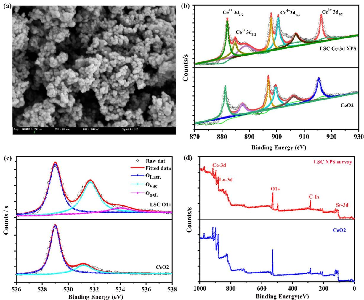
Fig. 4 (a) SEM image of  $\text{La}_{0.15}\text{Sr}_{0.05}\text{Ce}_{0.8}\text{O}_2$  powders. (b–d) X-ray photoelectron spectra of LSC and  $\text{CeO}_2$  corresponding high-resolution XPS spectra of Ce-3d, O 1s, and the XPS survey, respectively.
