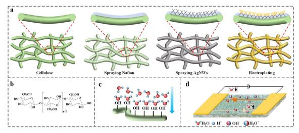
Fig. 3 (a) Schematic diagram of electrode adhesion to the paper. (b) Molecular formula of cellulose. (c) Schematic diagram of absorption of water molecules by –OH. (d) Schematic diagram of the sensing mechanism.
