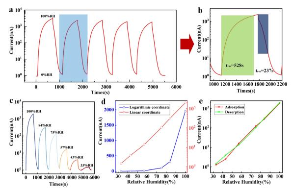
Fig. 5 Humidity-sensing properties of the humidity sensor. (a) Response and recovery curves for five cycles from 0% RH to 100% RH. (b) Amplified response and recovery curve. (c) Dynamic response characteristics curve of humidity sensor from 0% RH to 100%, 84%, 75%, 57%, 43%,33% RH. (d) Current–RH curves in logarithmic and linear coordinates. (e) Humidity response in adsorption and desorption state.
