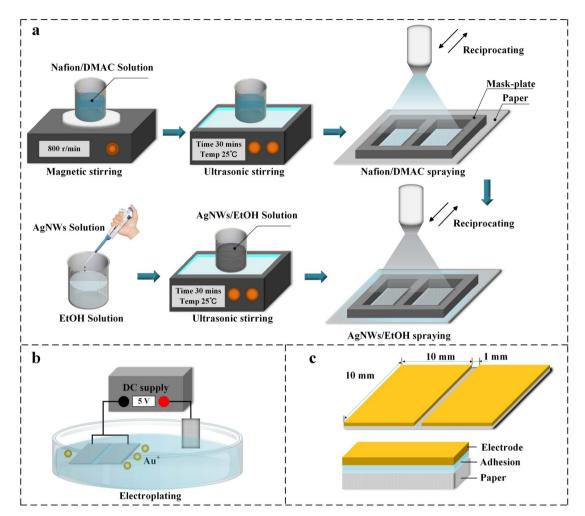
Fig. 1 The process of preparing the paper-based humidity sensors. (a) Preparation of the solution and process of spraying. (b) Process of electroplating (EP). (c) Schematic structure of the prepared sample.
