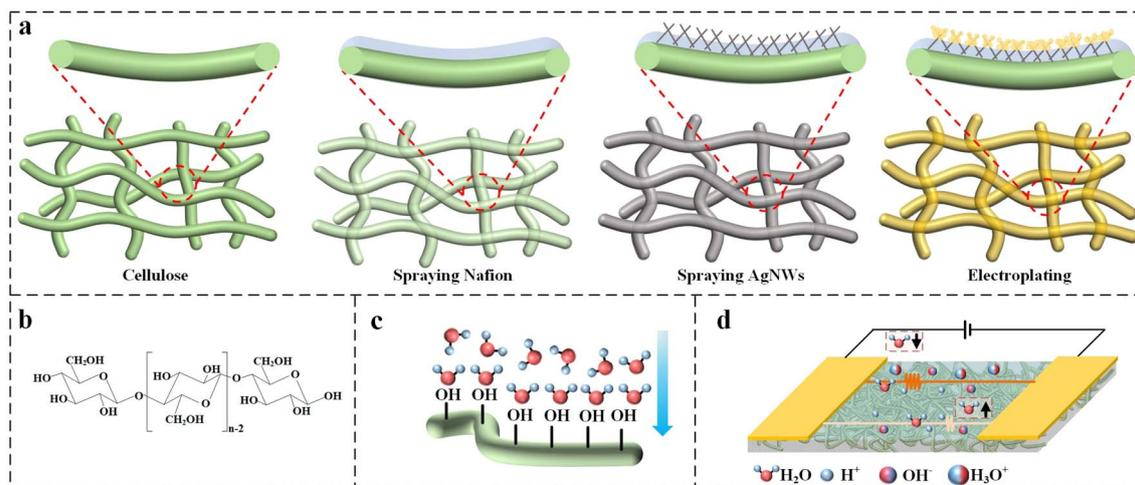
Fig. 3 (a) Schematic diagram of electrode adhesion to the paper. (b) Molecular formula of cellulose. (c) Schematic diagram of absorption of water molecules by  $-OH$ . (d) Schematic diagram of the sensing mechanism.
