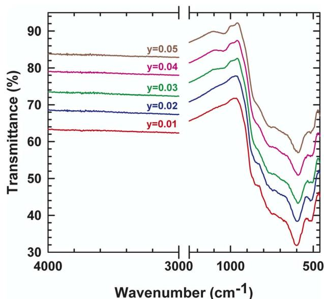
Fig. 5 IR spectra of  $\text{La}_2\text{Mo}_{2-y}\text{P}_y\text{O}_{9-y/2}$  ( $y = 0.01, 0.02, 0.03, 0.04, 0.05$ ).
