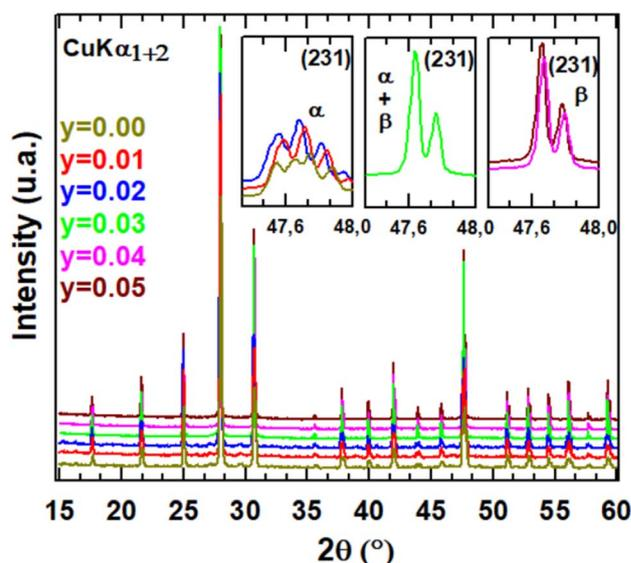
Fig. 1 Room temperature XRD patterns for different compositions of  $\text{La}_2\text{Mo}_{2-y}\text{PyO}_{9-y/2}$  series. The insets show the disappearance of the monoclinic splitting upon phosphorus substitution through the evolution of the (231) pseudocubic lines.
