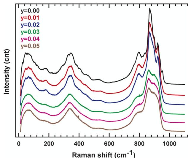
Fig. 4 Raman spectra of  $\text{La}_2\text{Mo}_{2-y}\text{P}_y\text{O}_{9-y/2}$  ( $y = 0.01, 0.02, 0.03, 0.04, 0.05$ ).
