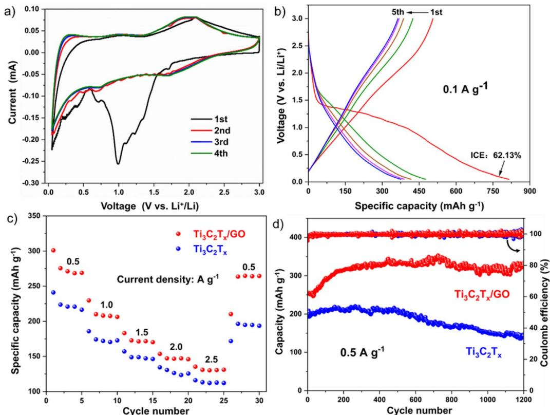
Fig. 6 (a and b) CV curve and charge–discharge curve of  $\text{Ti}_3\text{C}_2\text{T}_x/\text{GO}$  composites; (c and d)  $\text{Ti}_3\text{C}_2\text{T}_x$  and  $\text{Ti}_3\text{C}_2\text{T}_x/\text{GO}$  composites multiplier properties and cycle properties.
