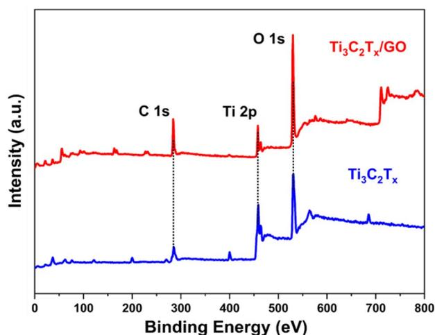
Fig. 4 XPS spectra of  $\text{Ti}_3\text{C}_2\text{T}_x$  and  $\text{Ti}_3\text{C}_2\text{T}_x/\text{GO}$  composites.
