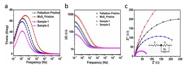
Fig. 6 EIS experiment data of MoS<sub>2</sub> pristine, different PdNPs@MoS<sub>2</sub> like sample-1 and sample-2 at OER onset potential, amplitude of 10 mV for the frequency range of 100 kHz to 0.1 Hz in 1.0 M KOH (a, b) Bode plots and (c) Nyquist plot.
