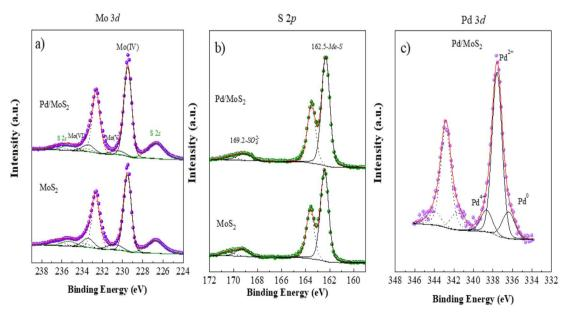
Fig. 4 XPS spectra of pristine MoS<sub>2</sub> and Pd doped sample-2 (a) Mo 3d, (b) S 2p, (c) Pd 3d.
