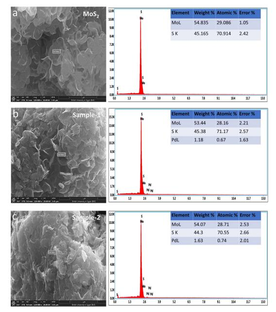
Fig. 2 SEM and EDS spectra of (a) MoS<sub>2</sub> pristine (b, c) sample-1 & sample-2.
