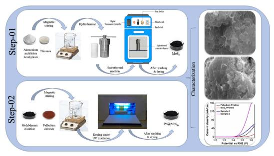
Scheme 1 Schematic view of palladium nanoparticles deposited on MoS<sub>2</sub> nanostructures
