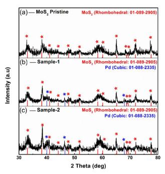
Fig. 1 Powder XRD diffraction of (a)  ${\rm MoS_2}$  pristine (b, c) sample-1 & sample-2.
