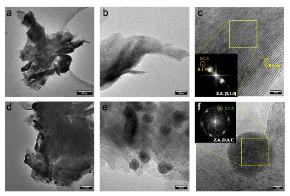
Fig. 3 TEM micrographs a different magnification of pristine  $MoS_2$  (a-c) and  $PdNPs@MoS_2$  (d-f). (c, e) HRTEM micrographs with inset illustrating the spatial frequencies of the crystallite displayed in the FFT.
