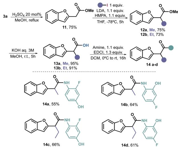
Scheme 4 Synthesis of  $\alpha$ -alkyl benzofuranyl acetic acid amides **14**.Table 1  $IC_{50}$  values against *Fusarium oxysporum* through mycelial growth inhibition
