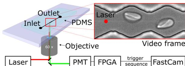
Fig. 1 Schematic of the microfluidic setup mounted on an inverted fluorescence microscope: RBCs entering the device and flow into the region of oscillating width and adopt their shape. Videos are taken with a fast camera and recording is triggered by cell passing a photoelectric barrier and rapid analysis in a photomultiplier tube.
