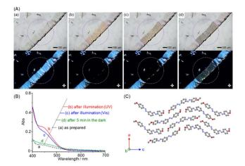
Fig. 2 (A) Optical microscopy images (top; bright field, bottom; under crossed polarizers) and (B) visible absorption spectra of drop cast film of 1 on a glass substrate. (a) As prepared, (b) after photoillumination with a mercury lamp (bandpass filter: 380-420 nm) for 5 s, (c) after photoillumination (bandpass filter: 510-560 nm) for 5 s, and (d) after standing for 5 min in the dark. (C) The crystal structure of (*E,E*)-1 along the *b*-axis.
