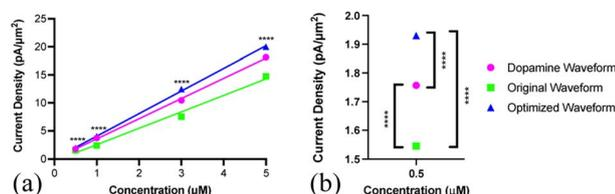
Fig. 5 (a) Calibration curves for Trp using three different waveforms (optimized MSW (green triangle), dopamine (magenta circle), and original MSW (blue square)). Error bars ( $\pm$ SEM) are too small to be visible. Only the  $t$ -test results comparing optimized vs. original waveforms are denoted in the graph. (b) Zoomed-in plot of the 0.5  $\mu\text{M}$  Trp showing how the optimized MSWs yielded higher current density than the dopamine and original waveform.  $****p < 0.0001$ .
