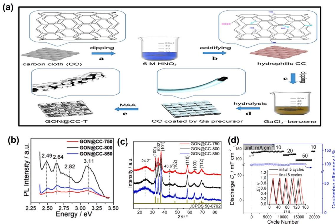
Fig. 6 (a) Synthesis procedure of GaON@CC-T. (b) Room-temperature PL spectra and (c) XRD spectra of GaON@CC-T ( $T = 750$  °C, 800 °C, and 850 °C). (d) Capacitance retention of the symmetric supercapacitor fabricated with GaON@CC-800 (these figures have been reproduced from ref. 31 with permission from Elsevier, copyright 2020) (the caption "GON" mentioned in the figure is the same as "GaON").
