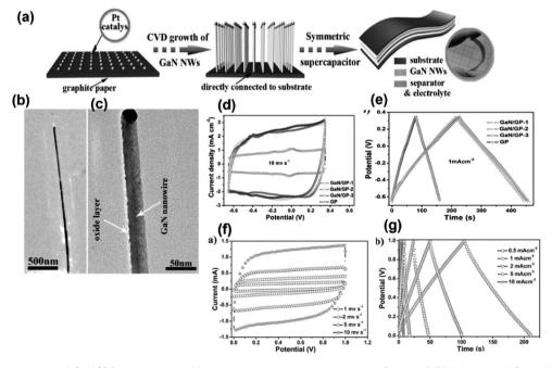
Fig. 4 (a) Synthesis process of GaN/GP and its assembly into symmetric supercapacitors. (b and c) TEM image of GaN NW. (d) CV graph at a sweep rate of 10 mV s $^{-1}$ . (e) GCD plot at a current density of 1 mA cm $^{-2}$  in the three-electrode set up. (f) CV curves and (g) GCD profiles of symmetric all-solid-state SCs fabricated by coupling hybrid GaN/GP-2 electrodes (this figure has been reproduced from ref. 26 with permission from Wiley, copyright 2002).
