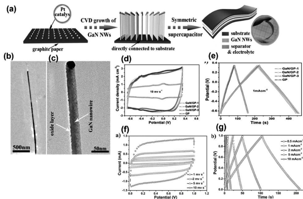
Fig. 4 (a) Synthesis process of GaN/GP and its assembly into symmetric supercapacitors. (b and c) TEM image of GaN NW. (d) CV graph at a sweep rate of  $10 \text{ mV s}^{-1}$ . (e) GCD plot at a current density of  $1 \text{ mA cm}^{-2}$  in the three-electrode set up. (f) CV curves and (g) GCD profiles of symmetric all-solid-state SCs fabricated by coupling hybrid GaN/GP-2 electrodes (this figure has been reproduced from ref. 26 with permission from Wiley, copyright 2002).
