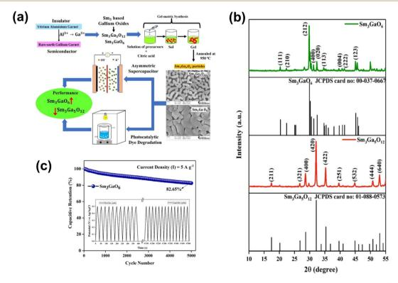
Fig. 10 (a) Synthesis process of  $Sm_3Ga_xO_y$ . (b) XRD spectra of  $Sm_3GaO_6$  and  $Sm_3Ga_5O_{12}$ . (c) Cycling stability curve of  $Sm_3GaO_6$  ((a–c) have been reproduced from ref. 43 with permission from RSC, copyright 2023).
