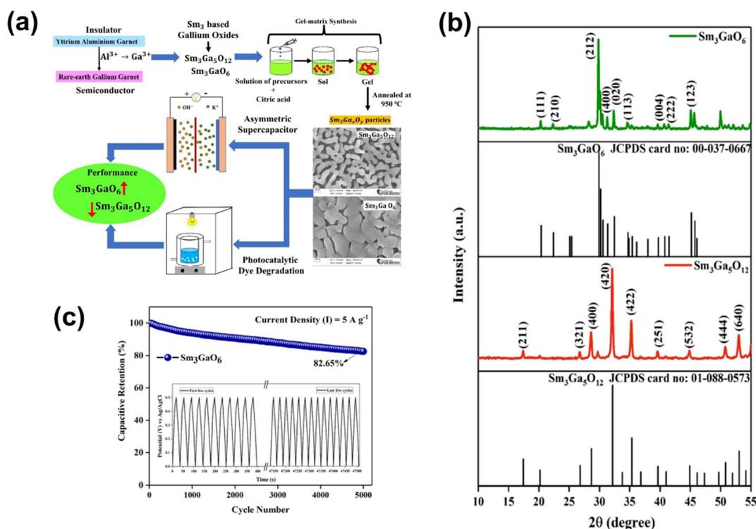
Fig. 10 (a) Synthesis process of Sm<sub>3</sub>Ga<sub>x</sub>O<sub>y</sub>. (b) XRD spectra of Sm<sub>3</sub>GaO<sub>6</sub> and Sm<sub>3</sub>Ga<sub>5</sub>O<sub>12</sub>. (c) Cycling stability curve of Sm<sub>3</sub>GaO<sub>6</sub> ((a–c) have been reproduced from ref. 43 with permission from RSC, copyright 2023).
