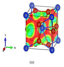
Fig. 9 (a) The (110) plane of V<sub>3</sub>Si and (b) the ELF with scale.
