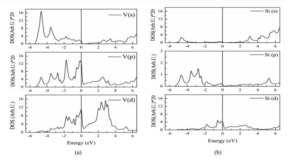
Fig. 2 Partial DOS from s, p and d states of (a) vanadium, (b) silicon atoms in  $V_3Si$ . To improve visibility the scale of DOS in case of V(s), V(p), Si(s) and Si(d) is multiplied by 20.
