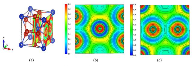
Fig. 8 (a) Crystal structure of  $V_3Si$  showing the (100) planes at x = 0.5 and x = 1 and the ELF. The enlarged views of the ELF in the two planes are shown in (b) and (c).
