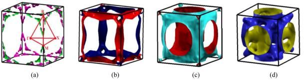
Fig. 3 The Fermi surfaces of V<sub>3</sub>Si from (a) first (b) second (c) third and (d) fourth band.
